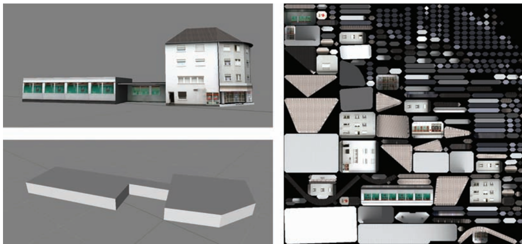
Figure 5-5: Visual mesh, physical mesh and texture of a building
