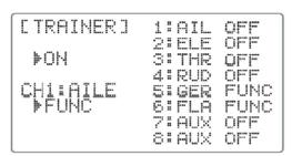
2. Since the FUTABA transmitters (especially the FF9/9C series), trainer switch is momentary switch, only if you leave it always "on" can realize its function. The simplest way for it is to hold the switch on with a rubber band. Other high-end transmitters such as (T9Z, T14MZ) have already put the trainer channel to always "on" Channel.
