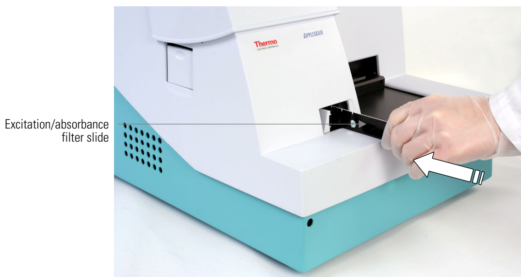
Figure 4–22. Inserting the excitation/absorbance filter slide
