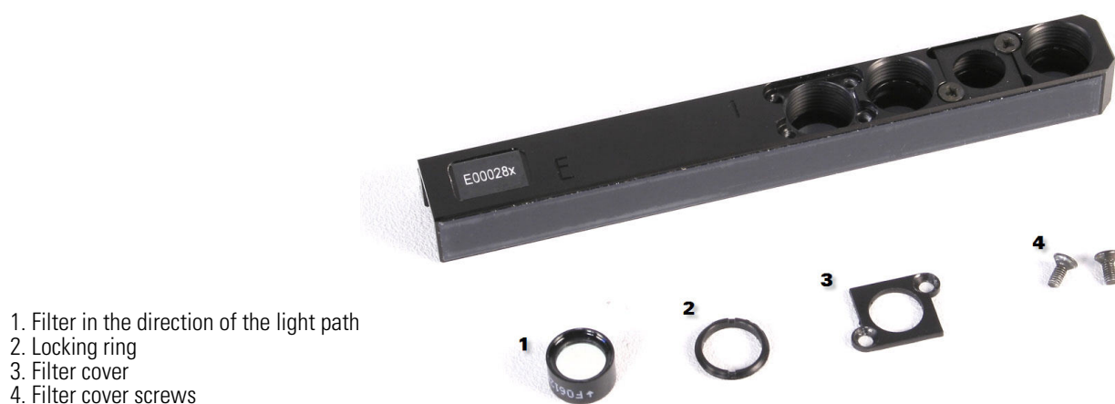
Figure 5–36. Parts of an excitation/absorbance filter slide
