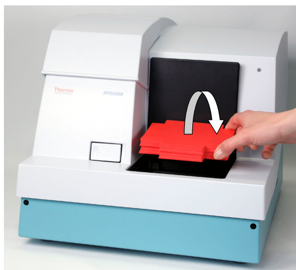
Figure 3–14. Removing the transport foam insert
