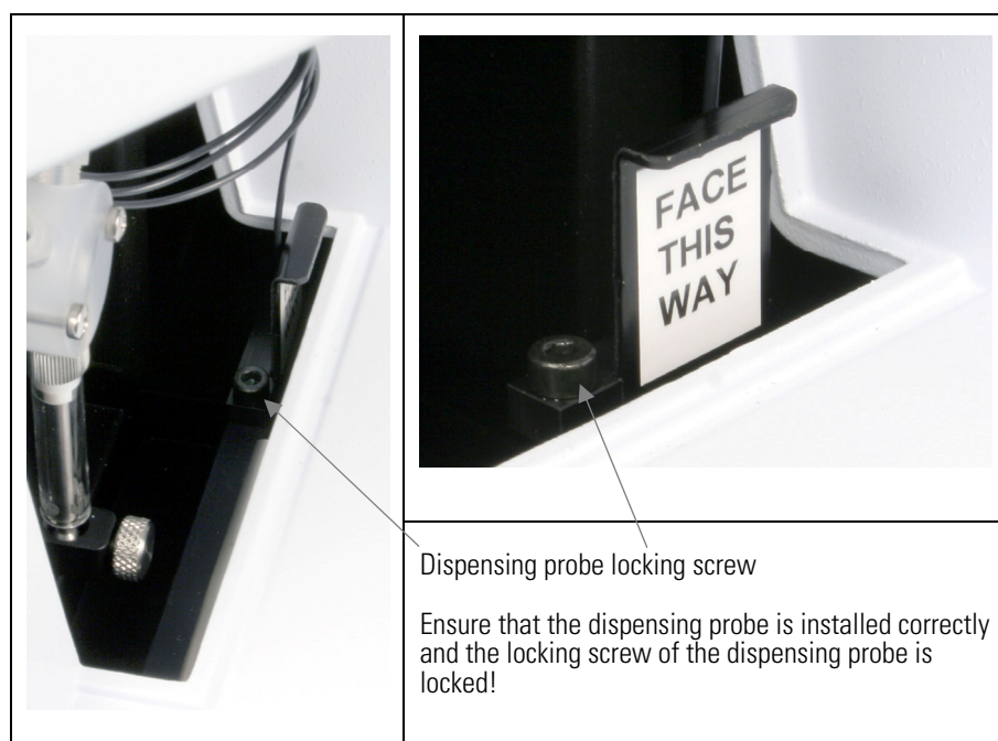
Figure 4–29. Replacing the locking screw of the dispensing probe
