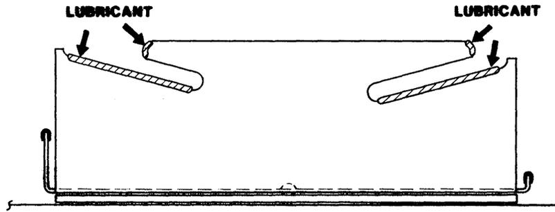
FIGURE 2-6. Control Unit Chassis Tilt/Swivel Assembly Lubrication
