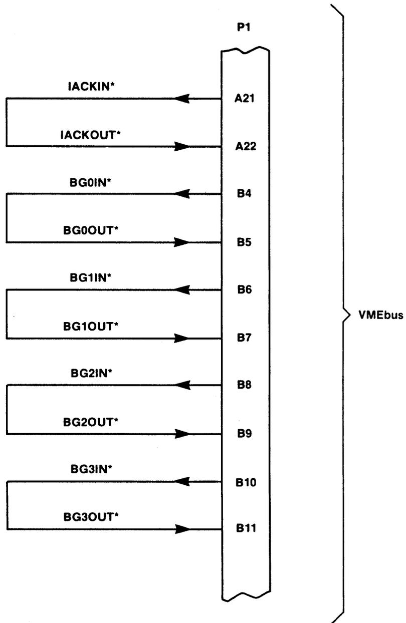
FIGURE 4-4. Typical VMEmodule Bus Arbitration Bypass
