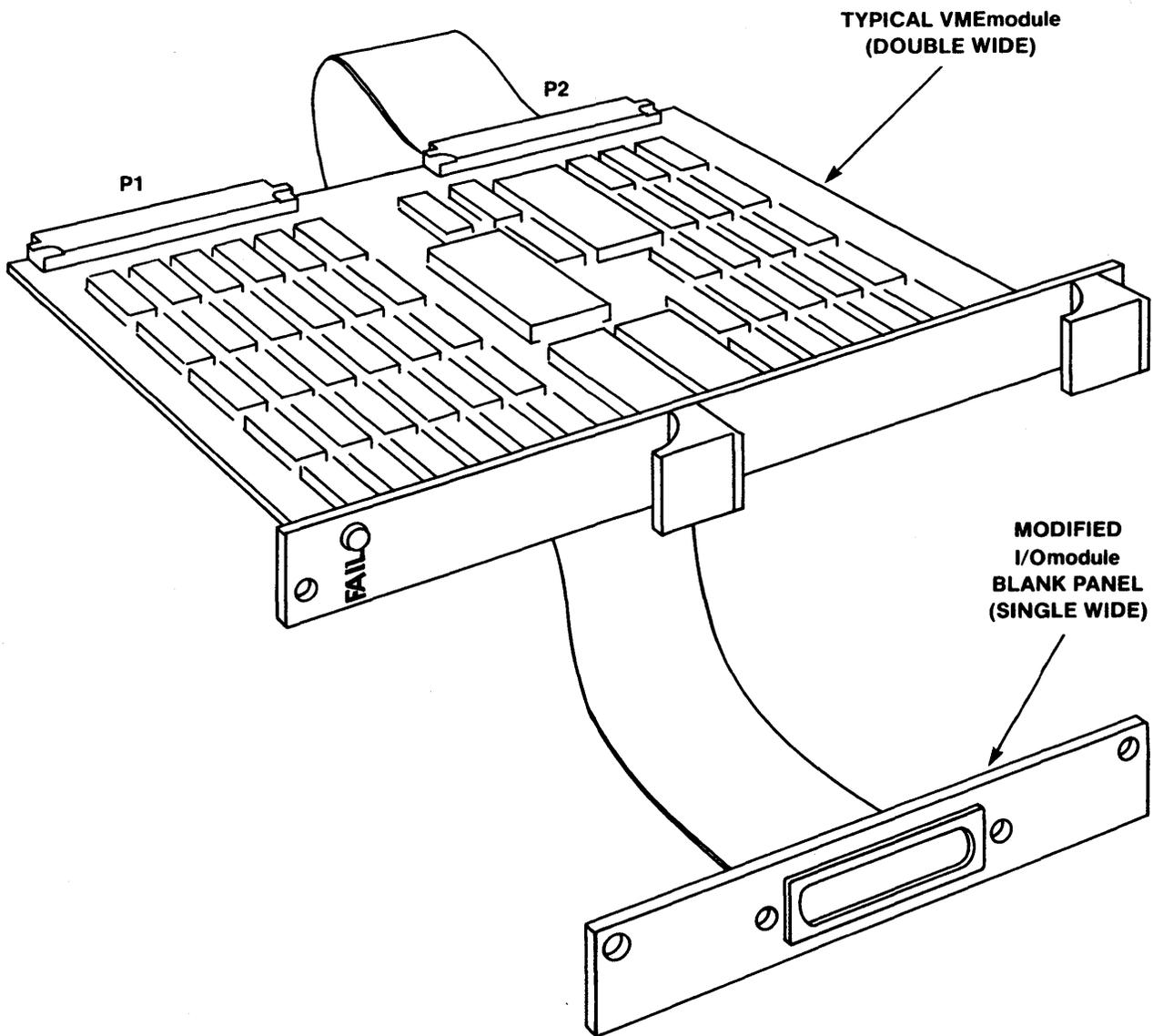
FIGURE 4-6. VME module I/O Cabling Method 1
