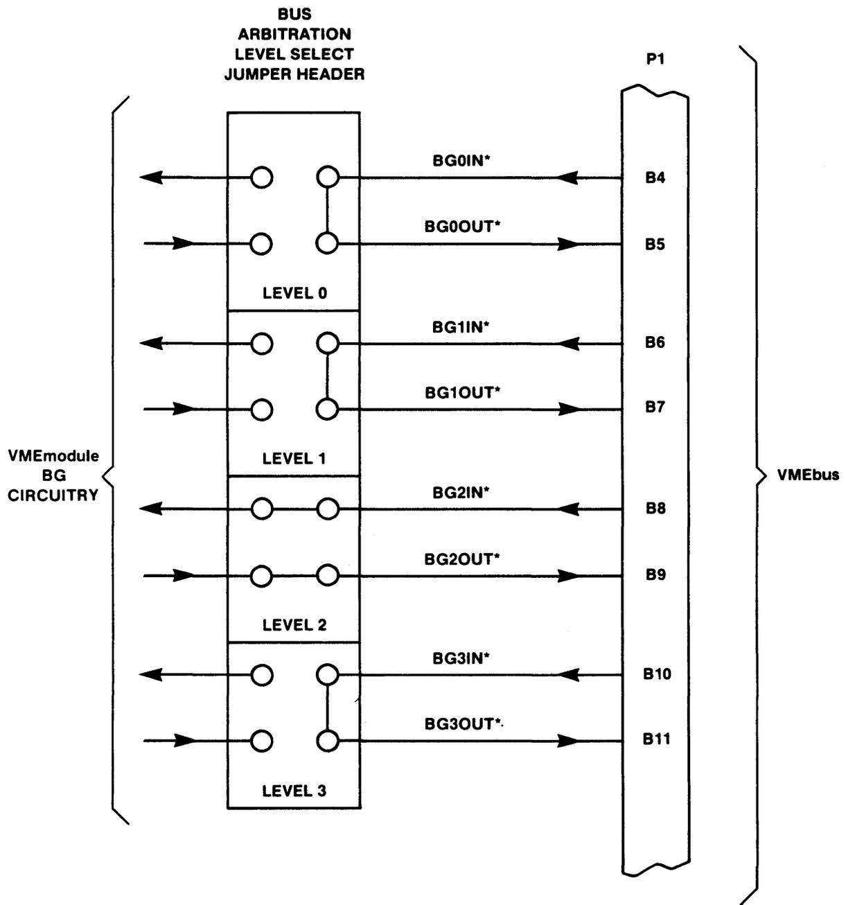
FIGURE 4-5. Typical VMEmodule Bus Arbitration Level Selection
