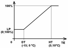
The parameters of ventilation time reduction are calculated automatically on the basis of the number of people, the walled area, the airtightness of the building and the calculation temperature.
