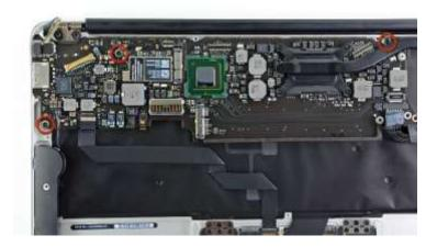
p. Gently lift the logic board assembly out of the upper case structure while being careful not to damage the fragile heat sink and any cables that may get caught
