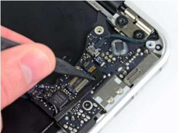
d. De-Route the left speaker cable from the notch cut into the small I/O board
