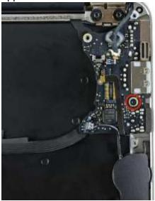
h. Carefully lift the I/O board from its edge nearest to the logic board and remove it from the upper case
