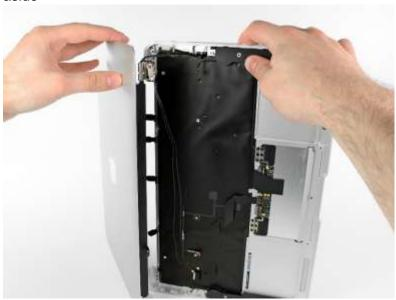
To re-assemble the machine into the attack configuration follow these steps in reverse. Any of the steps that involve re-attachment of connections to the display or modules in the display can be safely ignored. You may also wish to remove the antenna from the base of the display which can be accomplished using a Dremel tool and a careful hand. You may wish to confirm the startup functionality before removing the display module.
