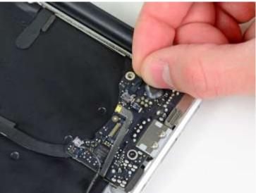
g. Remove from the small I/O board the single 3.6mm T5 Torx screw securing it to the upper case
