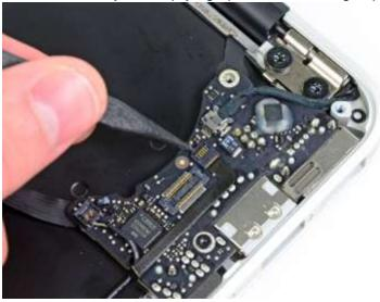
c. Pull the microphone ribbon cable straight out of its socket
