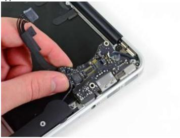
i. Peel up the six cable loops used to secure the antenna cables to the upper case
