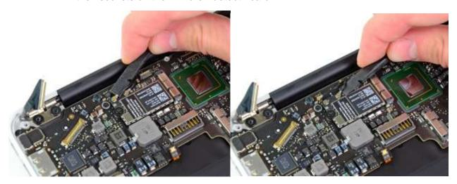
n. Gently de-route the antenna cables from the slot cut into the logic board
