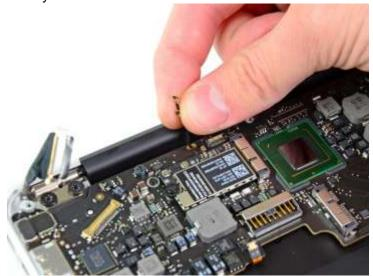
o. Remove from the logic board three 3.6mm T5 Torx screws used to secure it to the upper case structure
