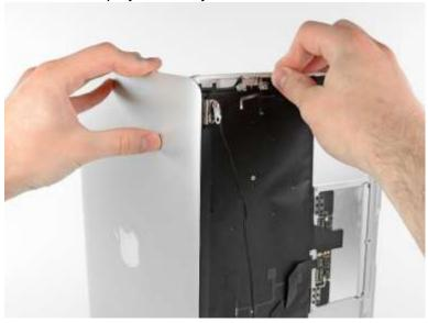
p. Once the two display hinges have cleared the upper case remove the display and set it aside
