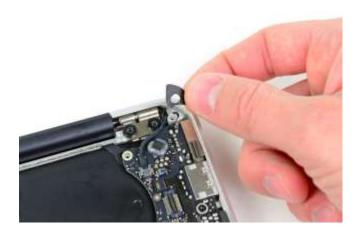
b. Use the pointed tip of a nylon spudge to carefully flip up the retaining flap on the microphone cable socket
