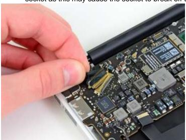
m. Use the flat end of the nylon spudger to pry both antenna cable connectors up and off their sockets on the AirPort/Bluetooth card
