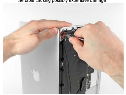
o. Push the upper case slightly toward the display assembly then rotate it away from the front of the display assembly
