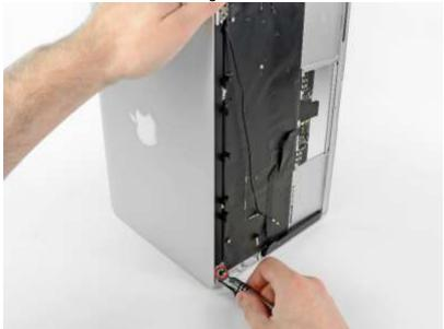
n. Remove the last 4.9mm T8 Torx screw securing the display to the upper case
