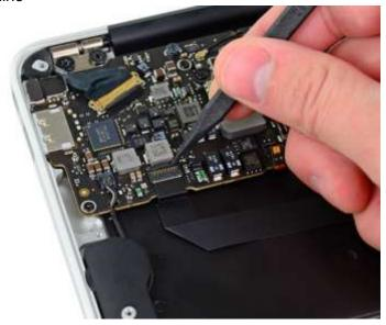
h. Use the point of the nylon spudger to de-route the right speaker cble from the slot cut into the logic board
