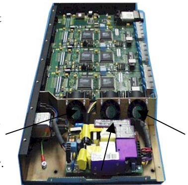
Figure 3.1: Location of the Magnum 6K25's cooling fans
