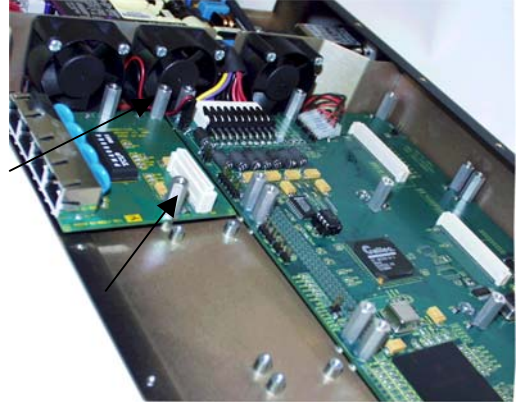
Fig 3.5.2b Granddaughter Board placed in slot A and secured with three 7/16 stand-off's
