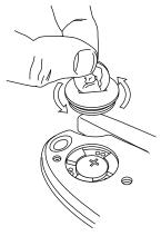
**2. Attach Mounting Bracket.** Attach mounting bracket to tripod thread.
