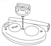
Secure to handlebar or strut using Velcro® strap. Fits bars 3/4" to 11/2" in diameter (19 to 38 mm).
