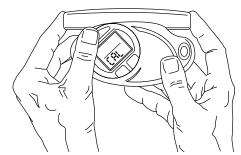
**Measure Wind Speed.** Point front of wind barrel into wind to measure positive (+) wind sped or headwind. Point rear of wind barrel into wind to measure negative (-) wind speed or tailwind.
