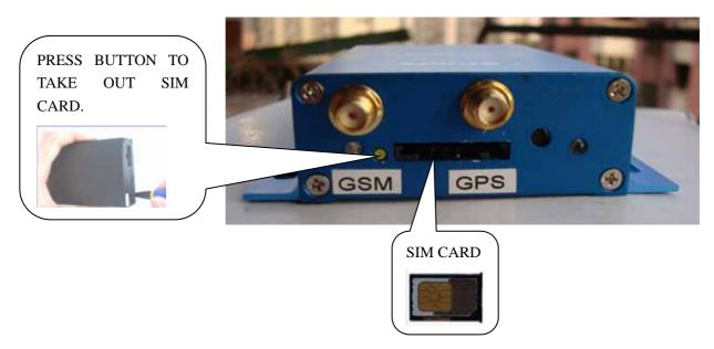
Insert the SIM card by Pressing the yellow hole ,the sim-card receiver will go outsie automatically -inset the sim-card
