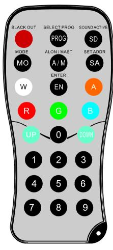
BLACK OUT: The lamp will be turned off after having pressed the button and exit to the status of Address Display. Press BLACK OUT+ 0 to reset to the initial status of infrared setting. (except address).
