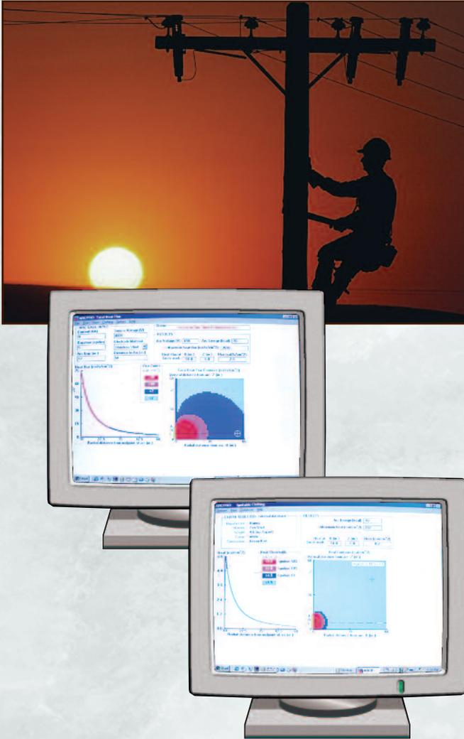
ARCPRO v.2 is a software program developed to calculate the thermal parameters of electrical arcs. The program is designed to aid in the selection of protective clothing by defining the arc hazard for workers who may be accidentally exposed to electrical arcs. The user can then specify clothing that will withstand the level of predicted arc hazards.
