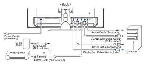
\* VGA (D-Sub) cable is not supplied with the monitor; you need to use a special VGA (D-Sub) cable dedicated for this model. Please contact the iiyama Support Centre in your country if you wish to connect the monitor via the VGA input.
