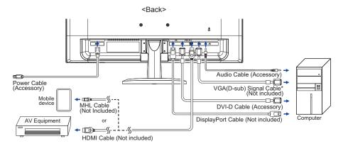
\* VGA (D-Sub) cable is not supplied with the monitor; you need to use a special VGA (D-Sub) cable dedicated for this model. Please contact the jivama Support Centre in your country if you wish to connect the monitor via the VGA input.
