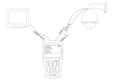
a. Press SET key to enter the sub-menu of PTZ controller.b. Press the or key to select the parameter
