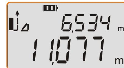
The meter calculates the distance A-B and displays it in the main display area.
