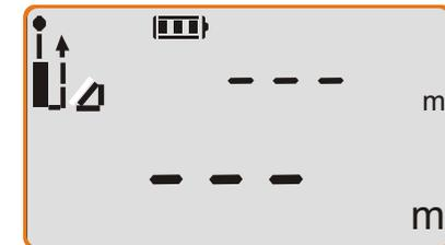
4. Aim the laser at the first measurement point (A) and press the ON/DIST button. The meter measures the distance: X-A, and displays it in the secondary display area.
