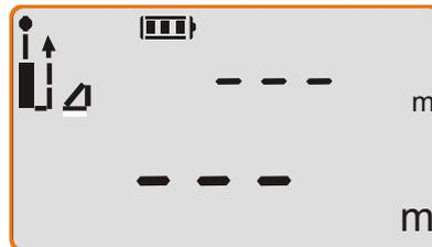
4. Aim the laser at the first measurement point (A) and press the ON/DIST button. The meter measures the distance: X-A, and displays it in the secondary display area.
