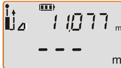
5. Moving the meter as little as possible, rotate it through 90° and point it at the second measurement point (B).
