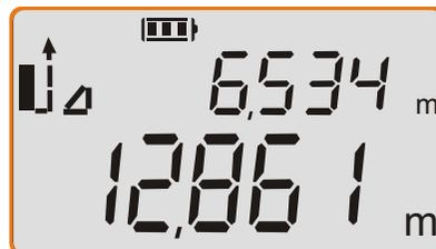
The meter calculates the distance A-B and displays it in the main display area.
