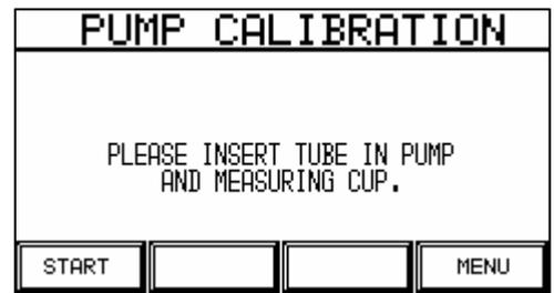
After starting calibration, the user is prompted to insert the tube into the pump and measuring beaker.
