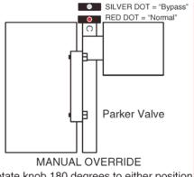
Rotate knob 180 degrees to either position Starting point - "C" stamped on valve body.
