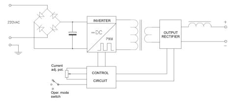
Figure 3 General electric diagram
