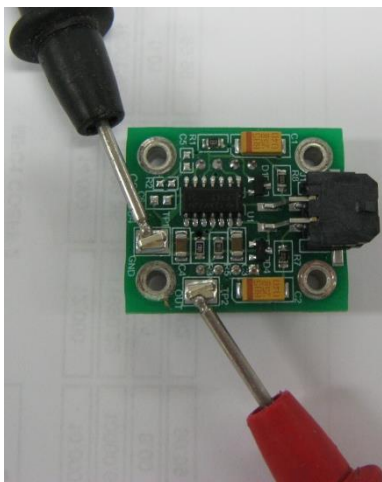
Figure 63 – Test Point Location
