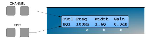
Pressing the edit navigation buttons gives access to the various pages of parameters available for each channel. The currently selected page is shown in the bottom left hand corner of the display, this is omitted on some pages where the function is obvious. The screen shows up to three (normally related) parameters for a given part of the processing functions on a given channel.
