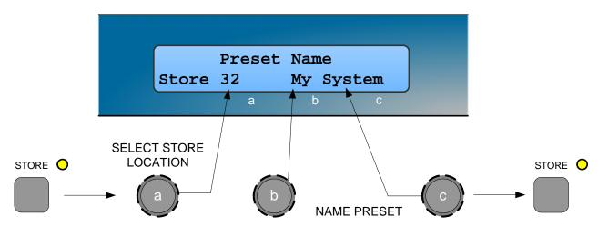
The user can overwrite non-protected Presets only; if an attempt is made to save a Preset in a location already occupied by a basic or Factory Preset a 'LOCKED PRESET' message is displayed.
