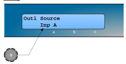
Knob A: Output source, selectable; Input A, Input B or Sum A+B
