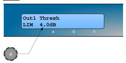
Knob A: Threshold, -40dBu to 20dBu in 0.2dB steps
