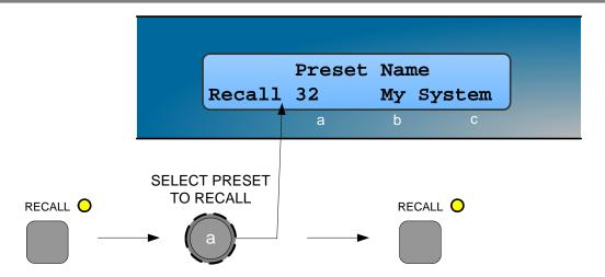
Users can develop their own Preset based on one of the Basic or Factory Presets stored within the device. Once a basic or user Preset has been recalled, a user has complete freedom to adjust any or all of the parameters. Factory Presets can be used as the basis for user Presets but they have some parameters that are predefined as a function of the loudspeaker system. These parameters are 'hidden' from the user, as they should be constant regardless of application.
