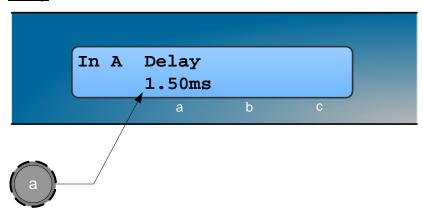
• Knob A: Delay, adjustable in variable steps from 0 to 400ms
