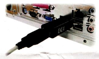
Please connect the USB key logger to your computer host and USB keyboard as above picture, it will start recording automatically.
