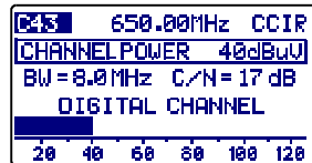
Figure 18.- Measuring a digital channel.
