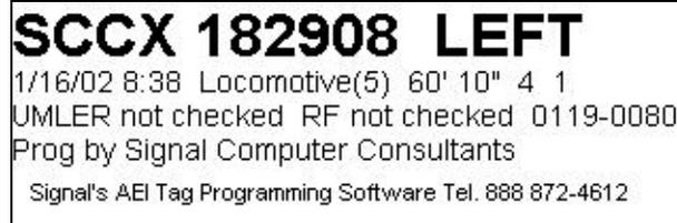
**Figure 14 - RF Not Checked Tag Label**
