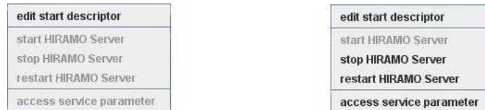
Figure 2.3: The control context menu for an RMI service, shown when the software system is not running (left) and when it is running (right).
