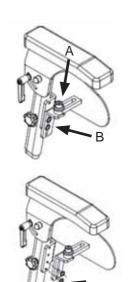
In addition to the height adjustment, hip support pads can be mounted in different heights to the armrest (C).
