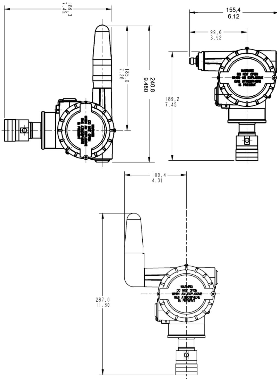
Figure 7—Typical mounting dimensions for in-line models STGW94L, STGW97L, STGW98L, and STGW99L (rear view)
