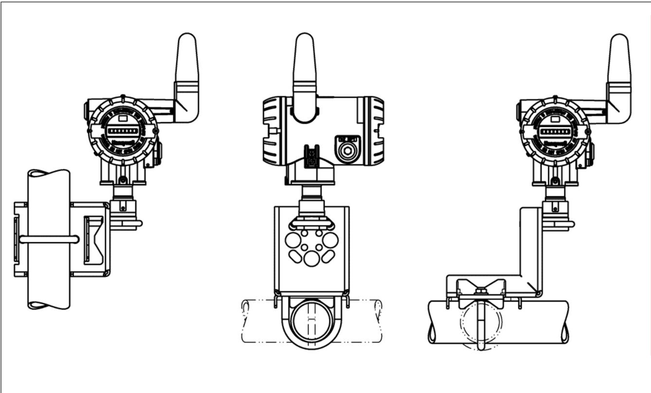
Figure 3 —Examples of typical mounting positions for in-line models STGW94L, STGW97L, STGW98L, STAW94L.
