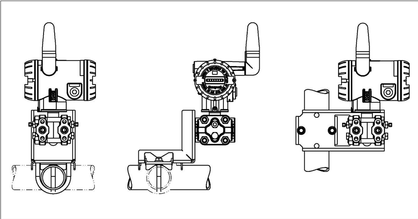
Figure 2—Examples of typical mounting positions for dual-head models STGW944 and STGW974
