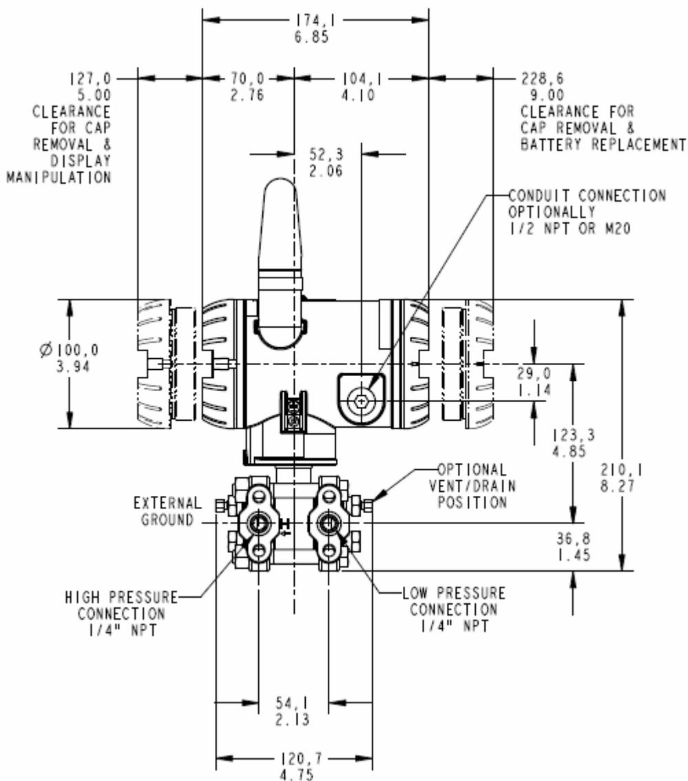
Figure 4 —Typical dimensions for dual-head models STGW944 and STGW974 (side view)
