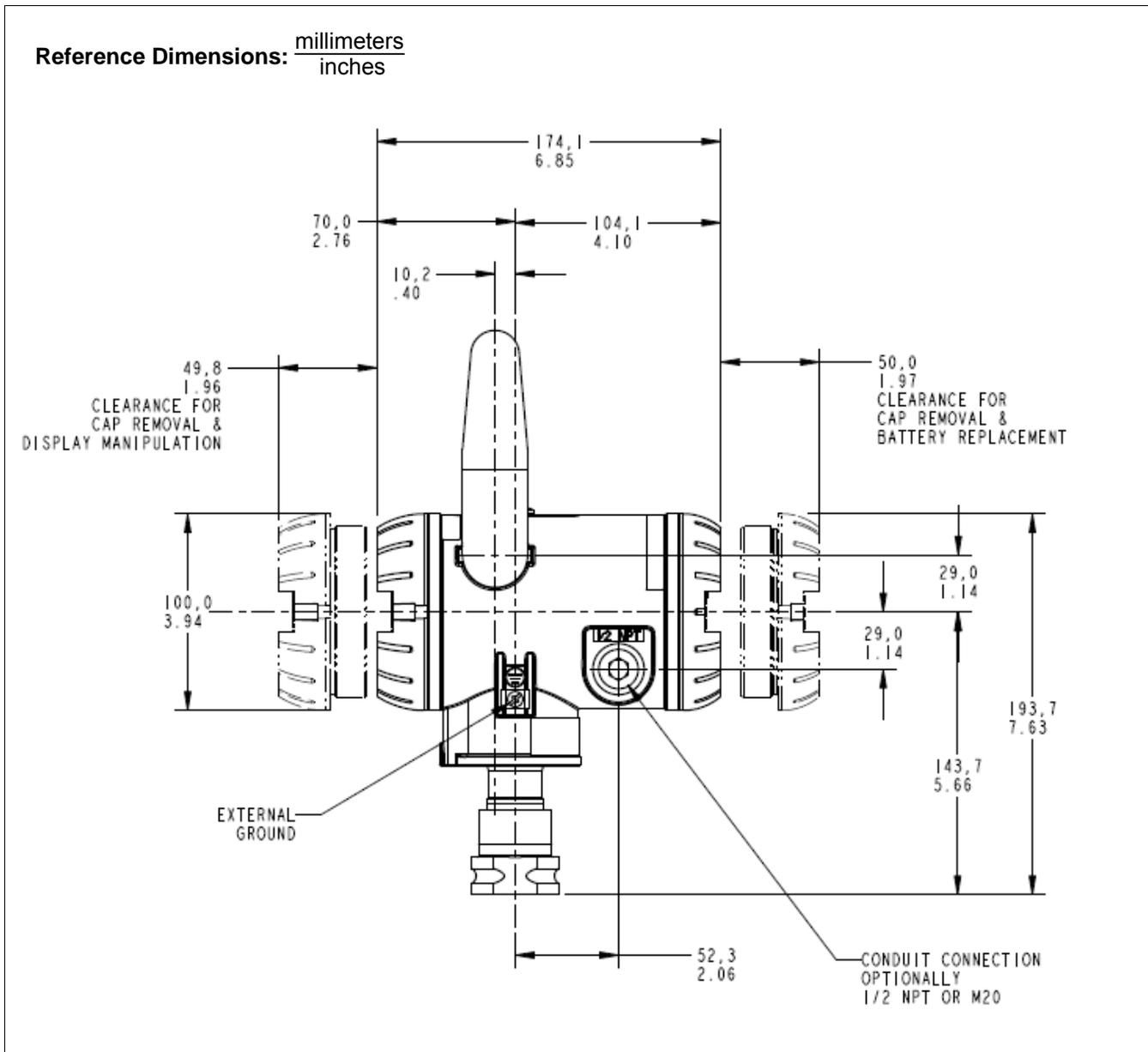
Figure 6—Typical mounting dimensions for in-line models STGW94L, STGW97L, STGW98L, and STGW99L
