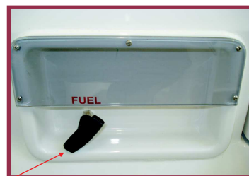
2. Emergency fuel cut off handle
