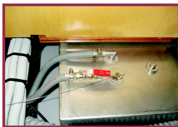
1. The fuel cut off valve
