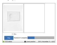
8 When the exposure is finished the image view appears displaying the image(s). You can navigate among the images by selecting the left or right arrows. You can also use the intensity tool to check pixel intensity.
