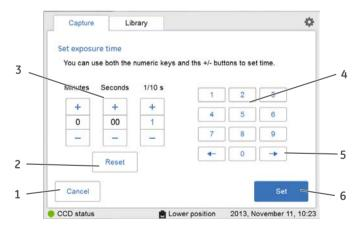
**Note:** The time displayed in the **Set exposure time** window, is by default the exposure time used during the last capture. The time can be set from 0.1 seconds up to 60 minutes.
