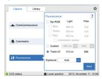
2 Check the *Epi-RGB* radio button, and then check the relevant detection channel check boxes of *Blue*, *Green and Red*.
