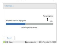
When the exposure is finished the image view appears displaying the images. Amersham Imager 600 creates a folder containing the created image files which can be saved. For details see *File formats, on page 126*.
