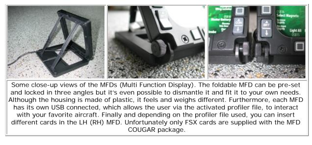
Finally but yet importantly, the slots on top of each display allows you to insert two Plexiglas windows where in-between you can insert the supplied FSX related cards or a decorative version. But what about the FS9 flight simmers?
