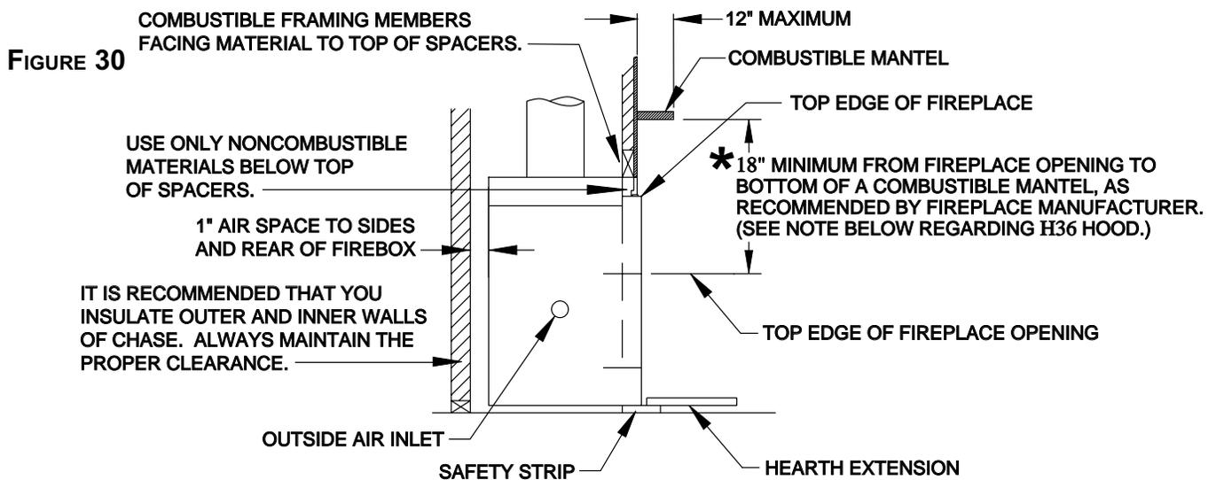
\* NOTE: IF AN APPROVED ANSI Z21.11.2 UNVENTED ROOM HEATER IS TO BE INSTALLED IN THIS FIREPLACE IN A RESIDENTIAL TYPE HOME, A MARTIN H36 HOOD MAY ALSO BE INSTALLED ON THE FIREPLACE TO REDUCE THE 18" RECOMMENDED CLEARANCE FROM THE TOP EDGE OF THE FIREPLACE OPENING TO THE BOTTOM OF A COMBUSTIBLE MANTEL TO 12" INSTEAD OF THE SPECIFIED 18".
