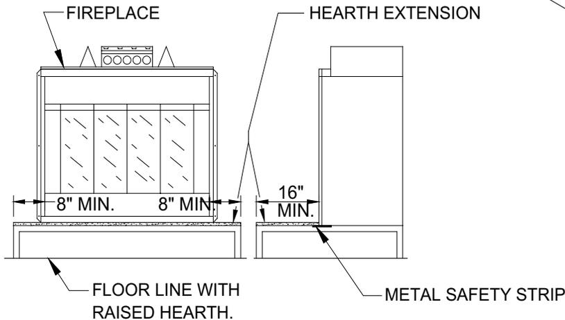
**WARNING:** THE HEARTH EXTENSION AND THE METAL SAFETY STRIP SHOULD BE INSTALLED ONLY IN A HORIZONTAL RELATIONSHIP TO THE FIREPLACE, AS ILLUSTRATED.
