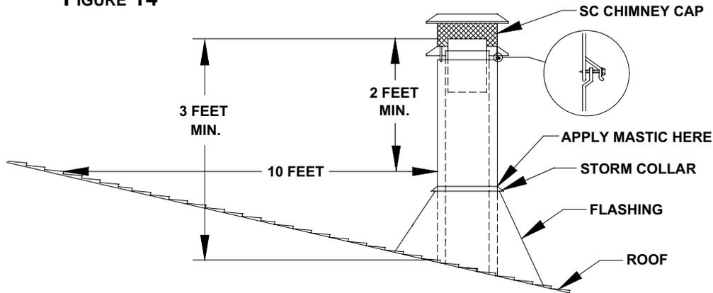
FOR SAFETY AND FOR PROPER DRAFT OPERATION, THE CHIMNEY MUST BE AT LEAST 3 FEET HIGHER THAN THE HIGHEST POINT WHERE IT PASSES THROUGH THE ROOF, AND IT MUST BE AT LEAST 2 FEET HIGHER THAN THE HIGHEST PART OF THE ROOF OR STRUCTURE THAT IS WITHIN 10 FEET OF THE CHIMNEY.
