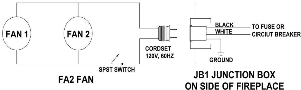
**NOTE: THE JBI JUNCTION BOX SHOULD BE INSTALLED AND ITS RECEPTACLE WIRED TO THE ELECTRICAL SYSTEM OF THE DWELLING DURING INSTALLATION OF THE FIREPLACE ON WHICH THE FA2 FAN IS TO BE UTILIZED.**
