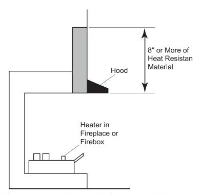
Figure 6 - Measuring Heat Resistant Material for Mantel
