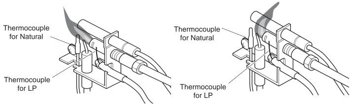
Figure 27 - Correct Appearance of Pilot Flame
