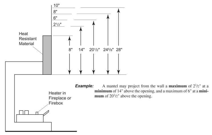
Figure 7 - Minimum Mantel Clearance with No Hood - DEB20
