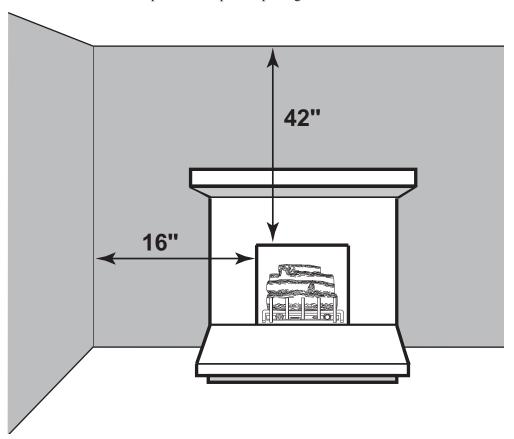
Figure 4 - Sidewall and Ceiling Clearances
