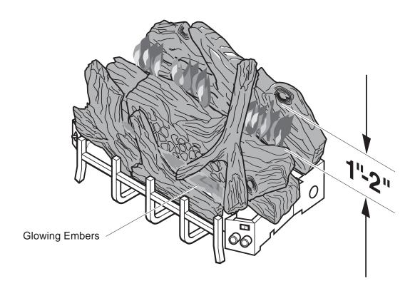
Figure 31 - Correct Appearance of Rear Flames
