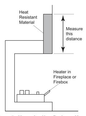
Figure 5 - Measuring Heat Resistant Material
