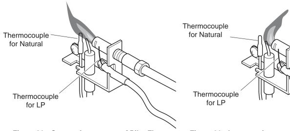
Figure 29 - Correct Appearance of Pilot Flame
