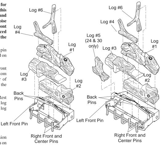
Figure 25 - Installing Logs to Grate (Model DEB20)
