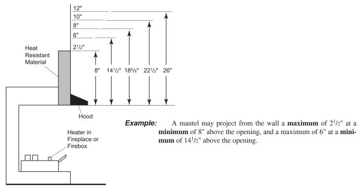
Figure 8 - Minimum Mantel Clearance with Hood - All Models
