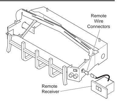
Figure 19 - Installing Remote Receiver
