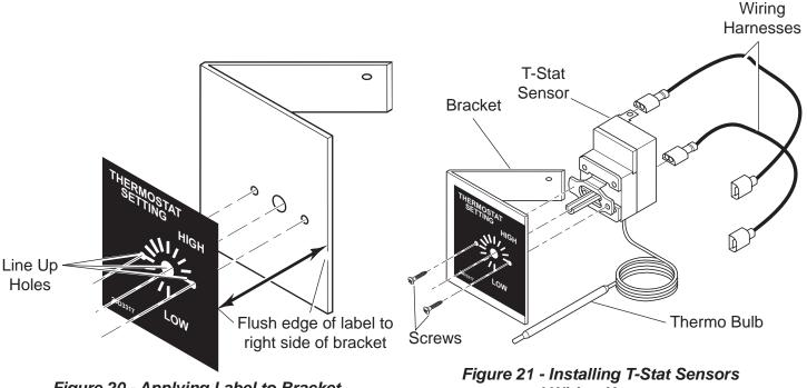
Figure 20 - Applying Label to Bracket
