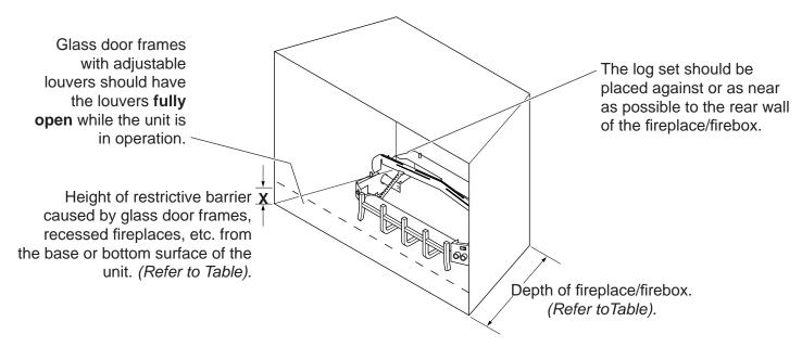
Figure 3 - Reference Drawing of a Natural Flame Log Set in an Enclosure
