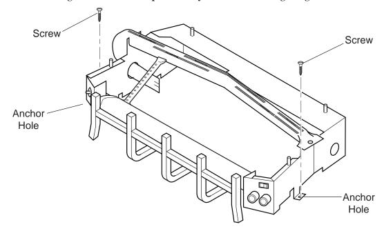
Figure 14 - Securing Heater to Floor of Fireplace/Firebox
