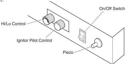
Figure 37 - Control Cover Plate for Milli-Volt
