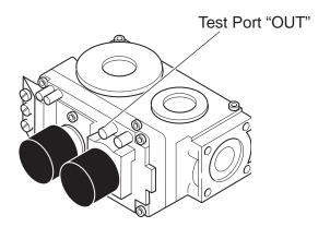
Figure 17 - Pressure Test Point Location Milli-Volt Control
