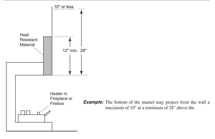
Figure 9 - Minimum Mantel Clearance with No Hood — DEB24 and DEB30
