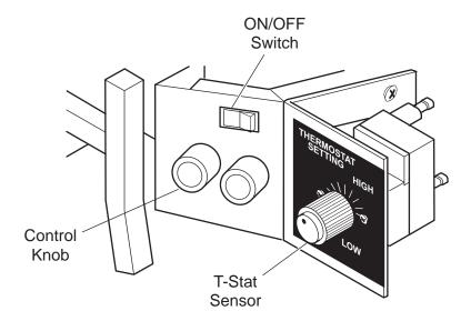
Figure 24 - Control Knob in "ON" Position and ON/OFF Switch in "OFF" Position
