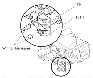
Figure 23 - Attaching Wiring Harnesses to Control Valve
