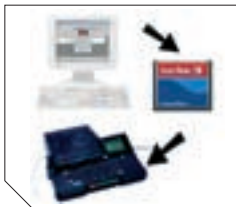
Transfer data files with marking information between the PC and the printer by using a compactflash memory.
