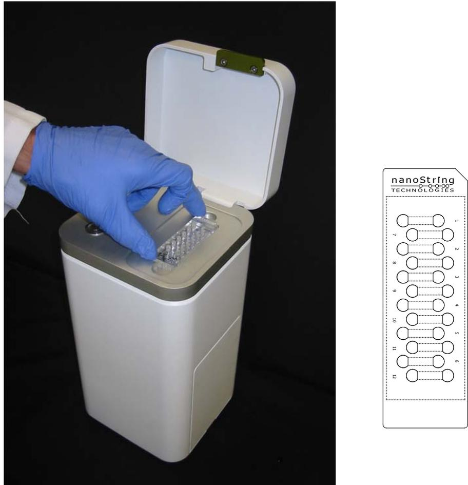
**Figure 3.25** nCounter Imaging Oil Applicator
