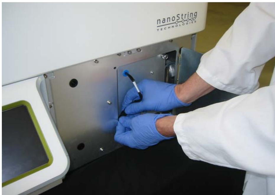
**Figure 3.11** Unplugging the Bulb Cable
