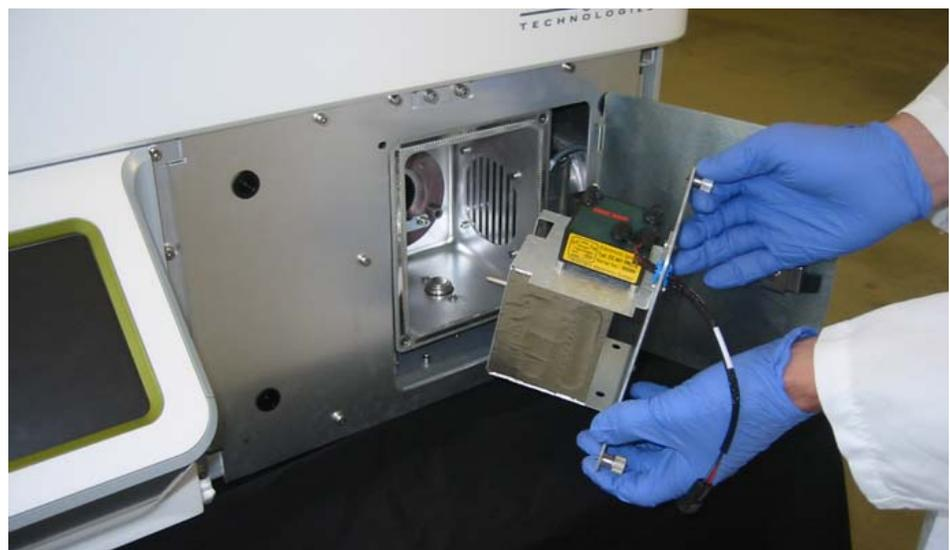
Figure 3.14 Inserting the Bulb Housing Unit
