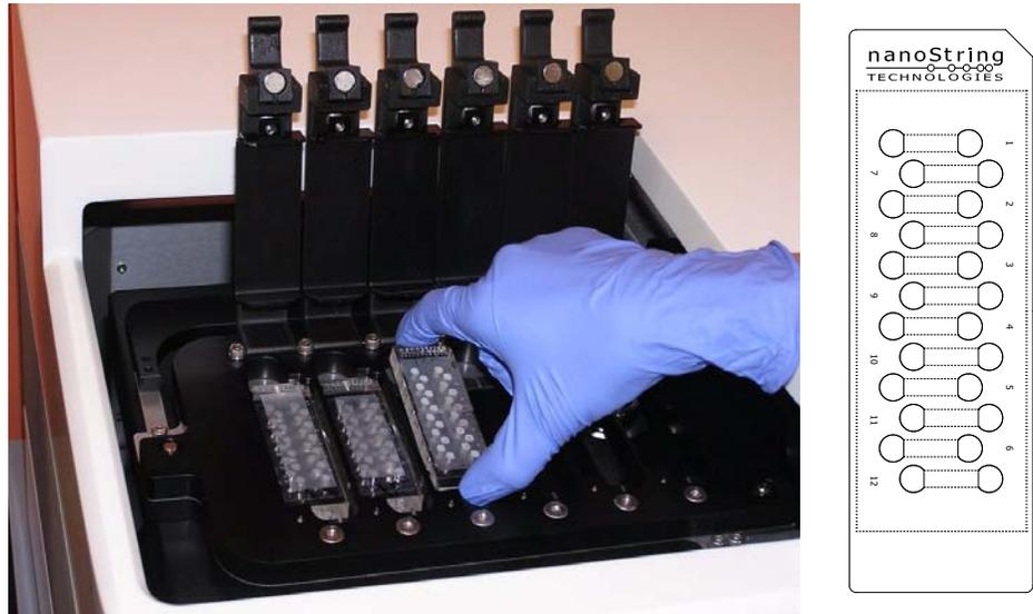
**Figure 2.30** Proper orientation of cartridges when placing them into the Digital Analyzer.
