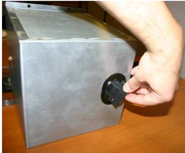
Figure 5-5 Pushing MDR-50 Connector through Grommet
