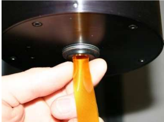
Figure 5-6 Gently Gripping the Flex Tether
