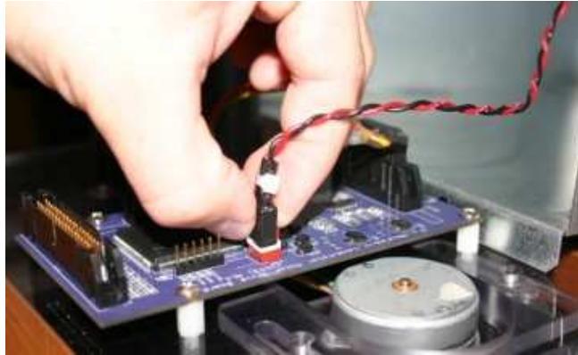
Figure 5-4 Removing the Power Connector
