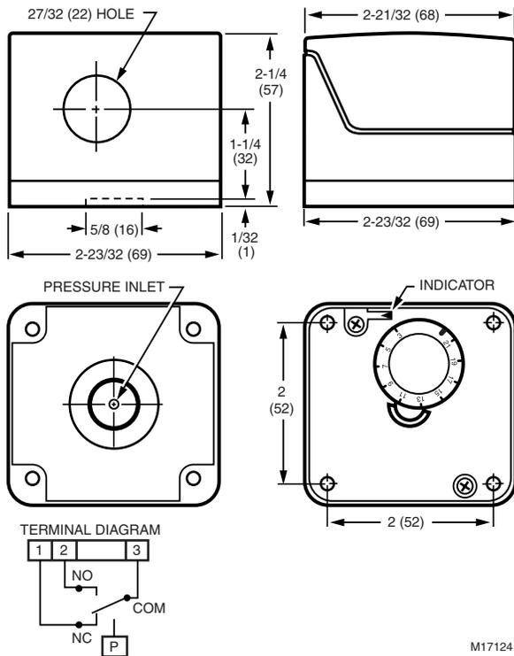
**Fig. 2. C6097 Flange Mount dimensions in in. (mm).**
