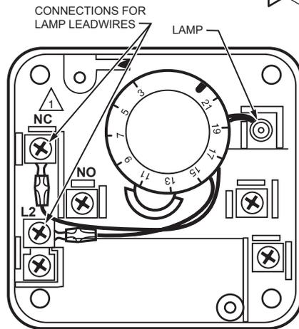
⚠ CONNECT L1 (HOT) LEAD TO THE NO OR NC TERMINAL BASED ON MODEL AND DESIRED LAMP FUNCTION.
