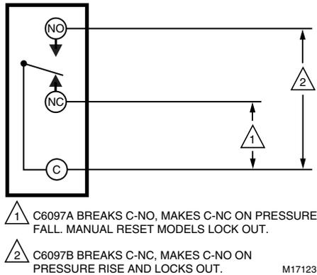
Fig. 9. C6097 schematic.
