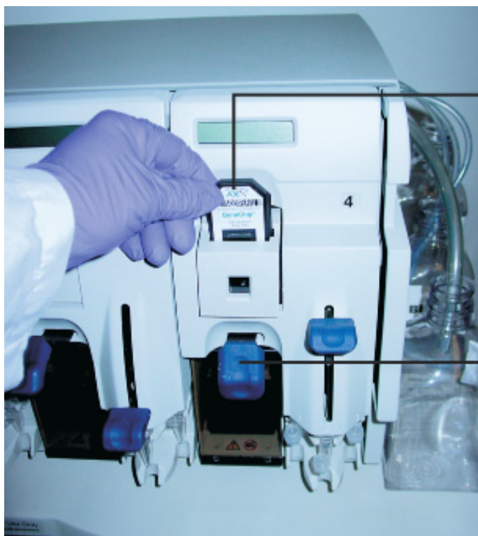
Figure 9.1 Disengaged Washblocks Showing Cartridge Levers in the Down Position. Remove any cartridges.
