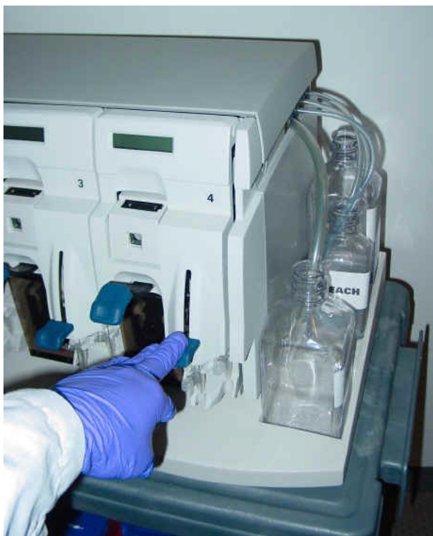
Figure 9.4 Press Down on the Needle Levers to Start the Bleach Protocol
