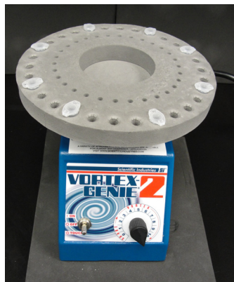
Figure 6.17 Resuspended Bead Clump and Vortexer with Foam Tube Adaptor
