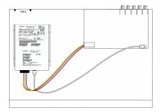
3) Affix HDD on HDD plate as indicated below with the screws around.
