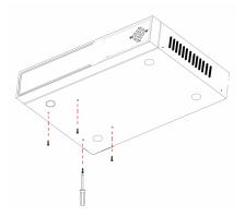
4) Install the HDD plate back into DVR and close cover .
