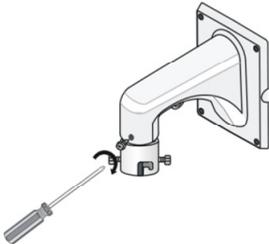
6. Lead the tail cable through the bracket, and push up.
