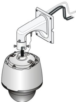
8. Hang the suspension loops in the concave of the conversion unit, and tighten 2 M5 screws.
