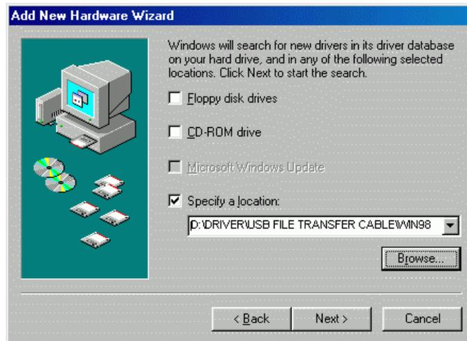
5.6 Windows® will detect the driver (**usbhc.inf**) and shows the **USB Bridge Cable**. Click **NEXT** to continue until installation is complete.
