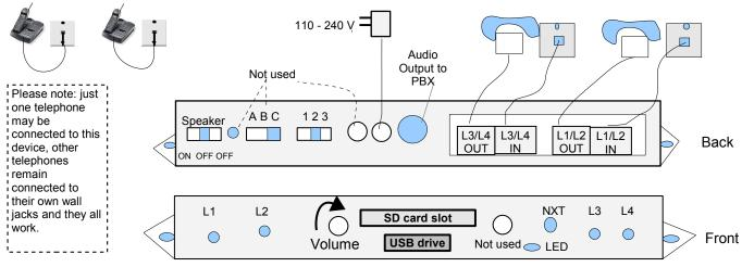
• Turn the Speaker ON to confirm Audio is playing and Adjust the Volume to mid level (you can Turn it OFF any time)
