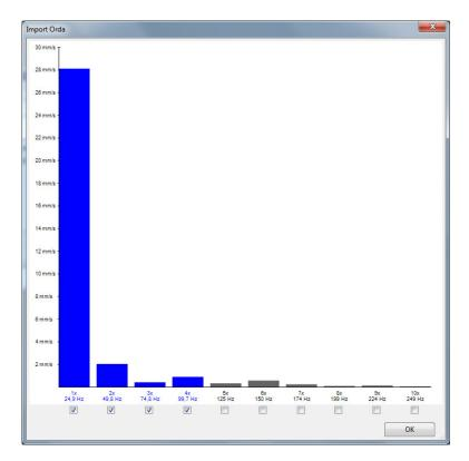
You can get the note that there are some undefined phases in imported animation set. This means that the VA4 analyzer did not measure some phases for certain Directions. The VA4 analyzer's result of measured phases on those directions was so unstable that there were saved as not measured in analyzer. It usually happens when the amplitude is very small. Press OK to continue.
