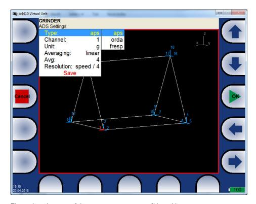
First select the type of the measurement you will be taking: aps – amplitude and phase on speed (you will need 1 acceleration sensor and tacho-probe) orda – order analysis (you will need 1 acceleration sensor and tacho-proble) fresp – frequency response (you will need 2 acceleration sensors)
