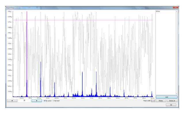
You can choose required frequency *By level*. In this case click to the Amplitude axis to choose the value and all frequencies with peak higher than the choice will be marked. You can select the Peak width from the choice on the bottom right part. By pressing *Add* you can add all of them at once. By dragging the gray borders of the graph you can specify the frequency band from which you wish to select the peaks. Press OK to confirm the selection.
