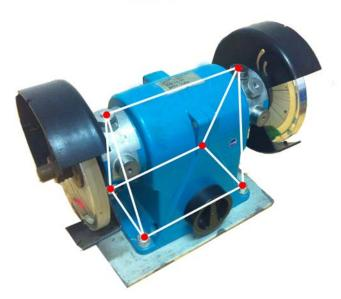
We need to move 2 existing points of our current square model to create bottom part of the grinder (rectangular) and add 2 more measurement points (to the top).
