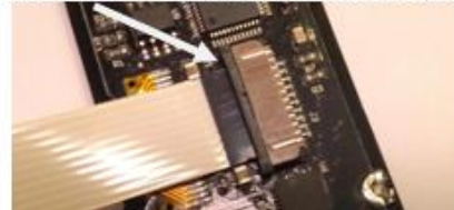
Close lock tab and fold ribbon cable as shown
