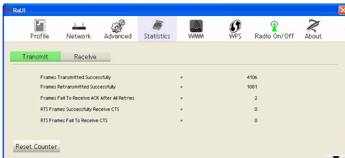
All connection-related statistics is displayed here. You can click the 'Transmit' or 'Receive' tab, to view the statistics of transmitted or received packets. You can also click the 'Reset Counter' button, to reset the statistics of all items back to 0.
