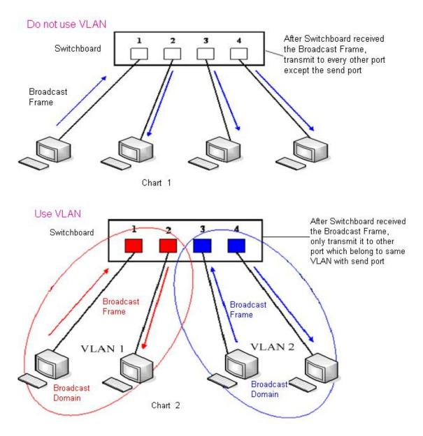
In chart 1, there is a layer 2 switch without setting VLAN. Any broadcast frame will be transmitted to the other ports except the send port. For example, a broadcast information is sent out from port 1 then transmitted to port 2,3and 4.
