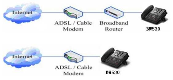
Shared network connection—Use this method if you have a single Ethernet port in your workspace with your desktop computer already connected to it. First, disconnect the Ethernet cable from the computer and attach it to the WAN port on the back of your phone. Next, use the Ethernet cable in the package to connect LAN port on the back of your phone to your desktop computer. Your IP Phone now shares a network connection with your computer. The following figure is for your reference.
