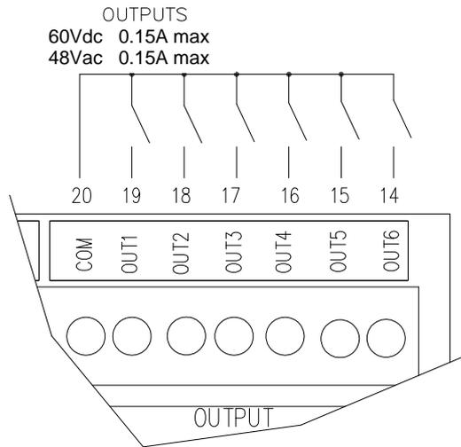
The maximum power of the photomofet outputs 48 Vac 0,15 A max (or 60 Vdc 0,12 A max),
