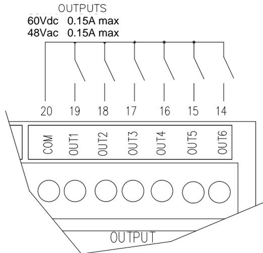
The maximum power of the photomofet outputs 48 Vac 0,15 A max (or 60 Vdc 0,15 A max).
