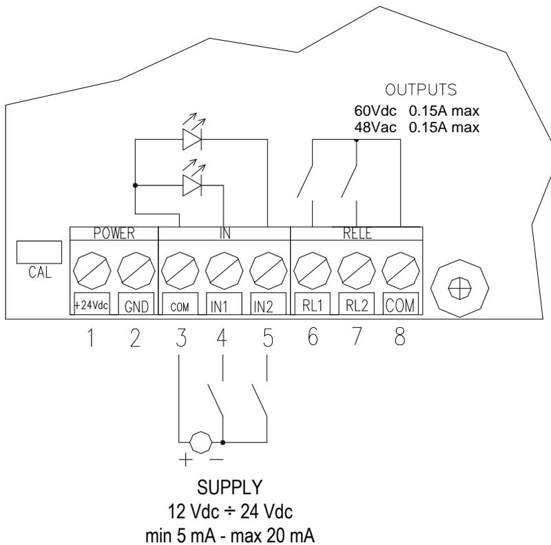
The maximum power of the outputs 48 Vac 0,15 A max (or 60 Vdc 0,15 A max), the maximum voltage applicable to the inputs is between 12 ÷ 24 Vdc with current from minimum 5 mA to maximum 20 mA.
