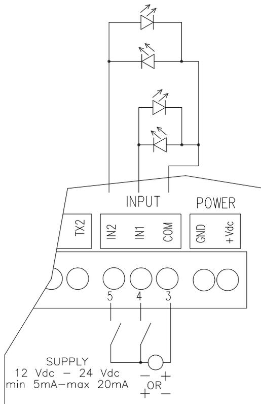
The maximum voltage applicable to the inputs is between 12 ÷ 24 Vdc with current from minimum 5 mA to maximum 20 mA.
