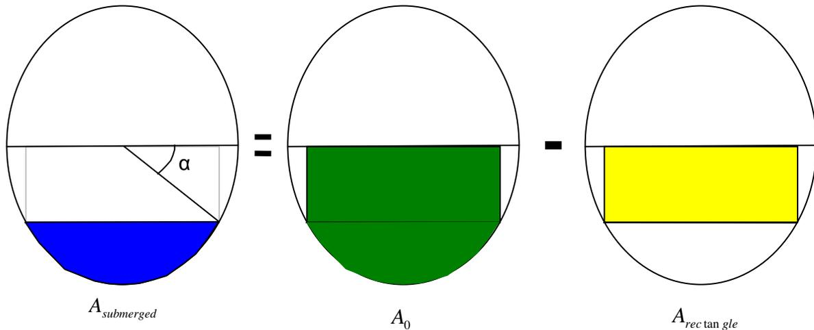
**Fig. 1.21 Description of fuselage submerged area ( $\alpha < 0$ )**
