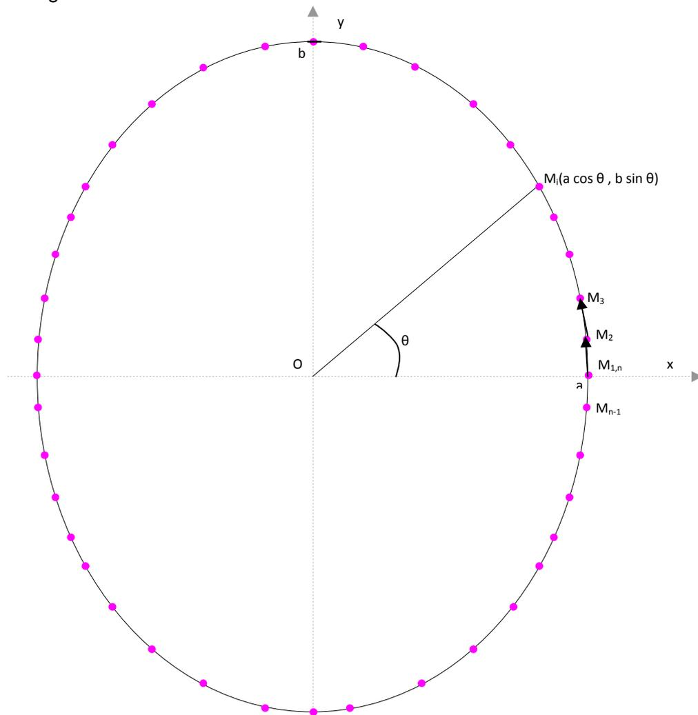
**Fig. 2.27 Points used to draw an ellipse**
