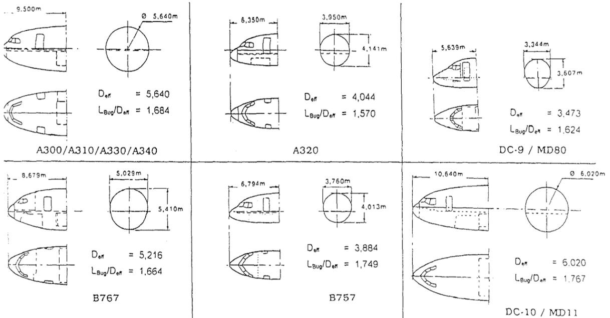
**Fig. 1.17** Nose length of existing airliners [Schmitt 1988]
