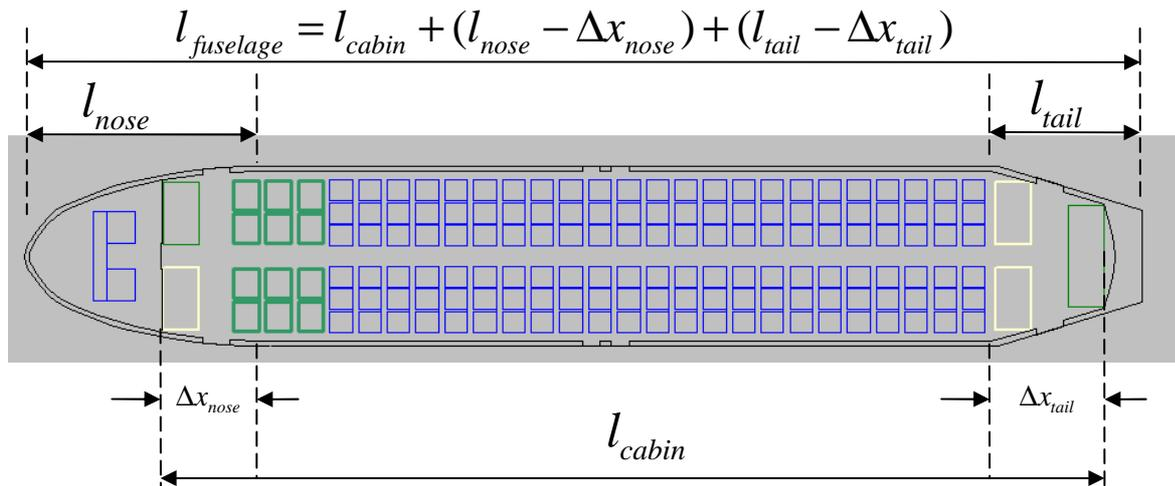
**Fig. 1.19 Calculation of the fuselage length**
