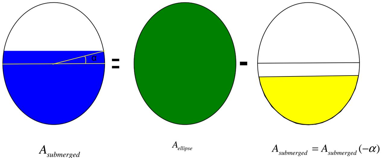
**Fig. 1.23 Description of the fuselage submerged area ( $\alpha > 0$ )**
