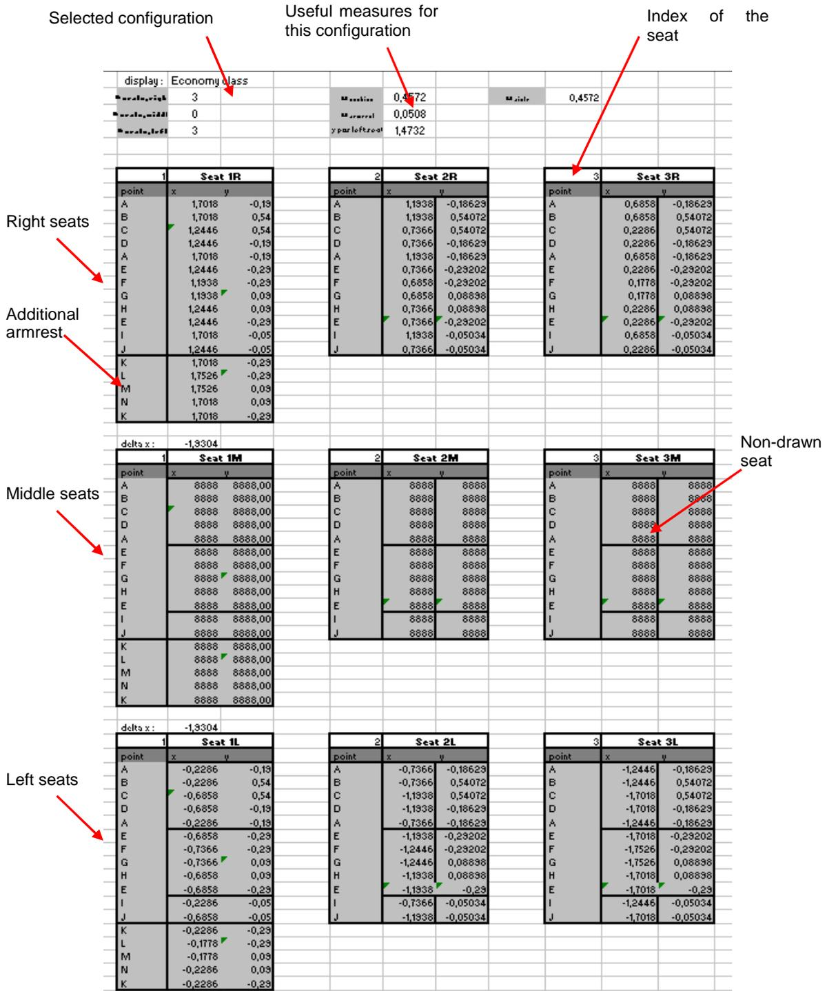
Fig. 2.34 Calculation of seats coordinates in cabin cross section
