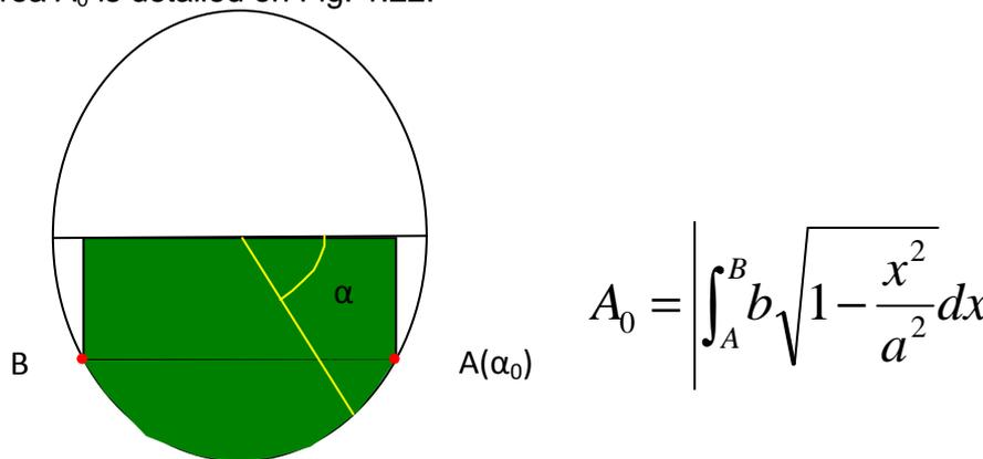
**Fig. 1.22 Area  $A_0$  used for waterline**
