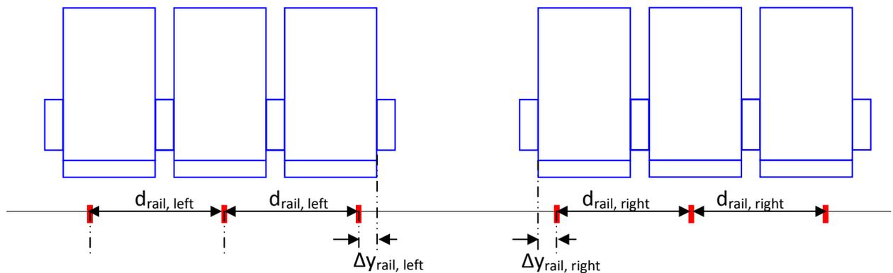
**Fig. 1.12 Positioning of seat rails on a single aisle**
