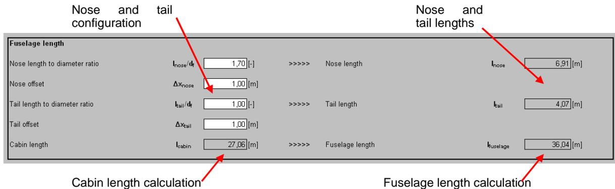
**Fig. 2.21 Calculation of fuselage length**
