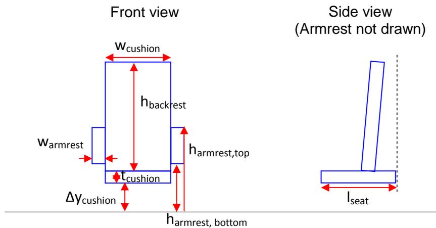
**Fig. 2.3 Definition of seat dimensions**
