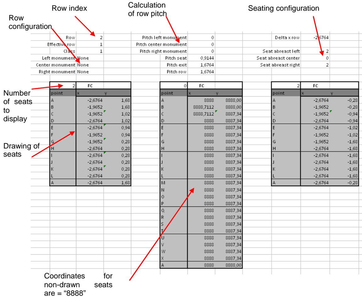
**Fig. 2.43 Calculation of seats position for the cabin floor plan**
