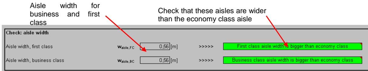
**Fig. 2.14 Check of aisles width**
