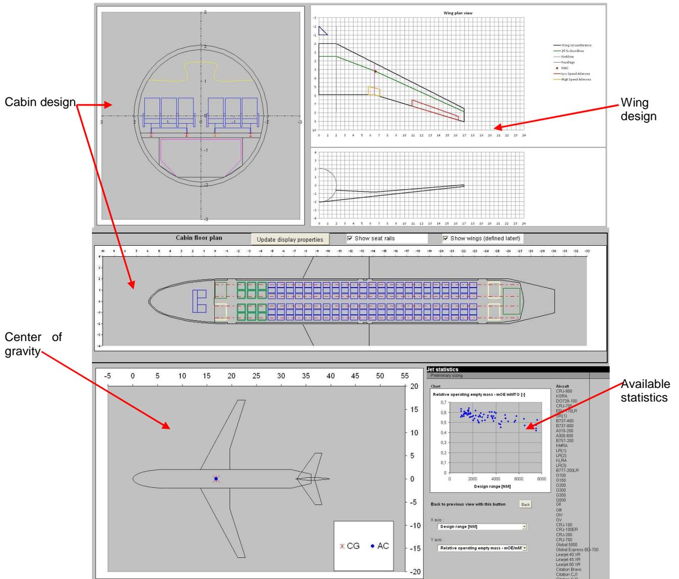
**Fig. 1.1 Design of an aircraft in PreSTo**
