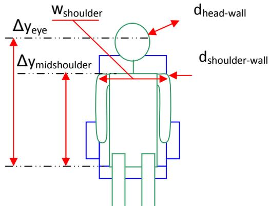
**Fig. 2.6** Definition of passenger dimensions
