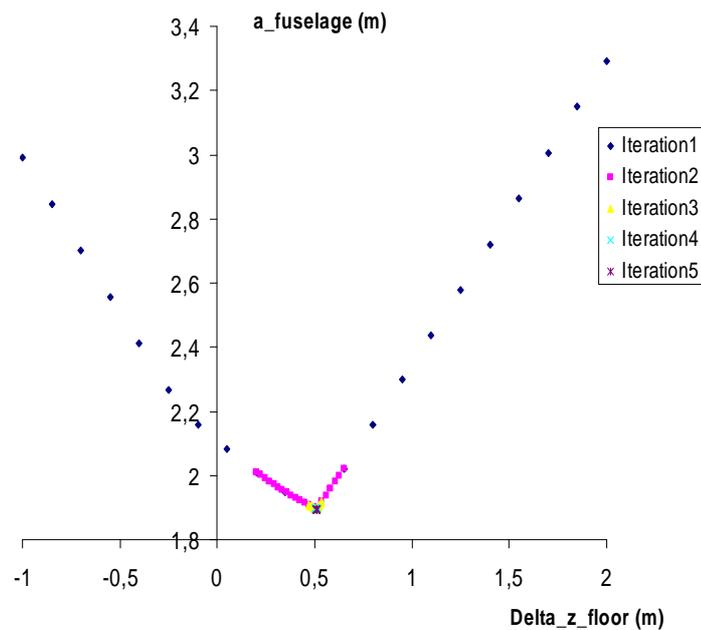
**Fig. 2.56** Evolution of fuselage semi height through five iterations
