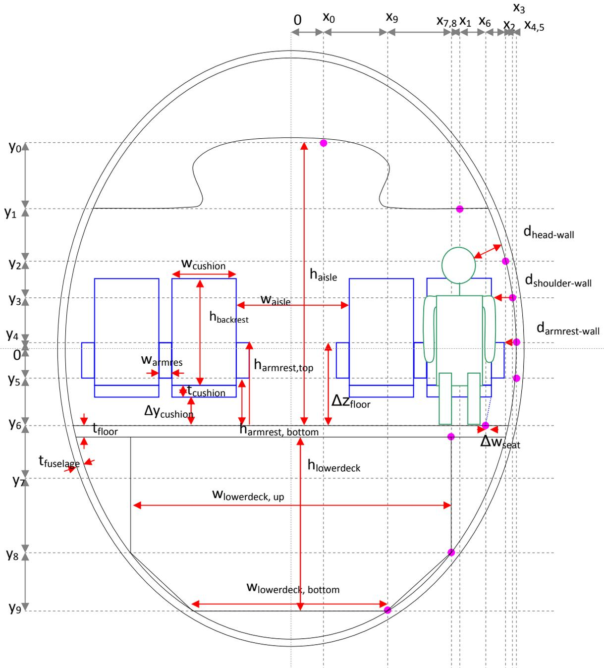
**Fig. 1.9 Definition of generic cross section of an aircraft as used in PreSTo-Cabin**
