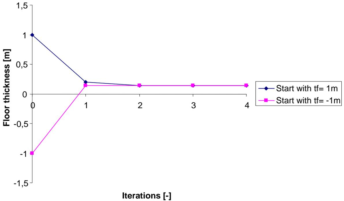
**Fig. 1.10 Evolution of floor thickness value through four iterations**
