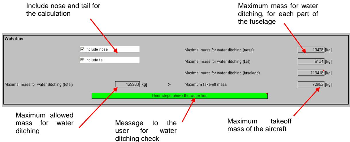
**Fig. 2.24 Calculation of waterline**
