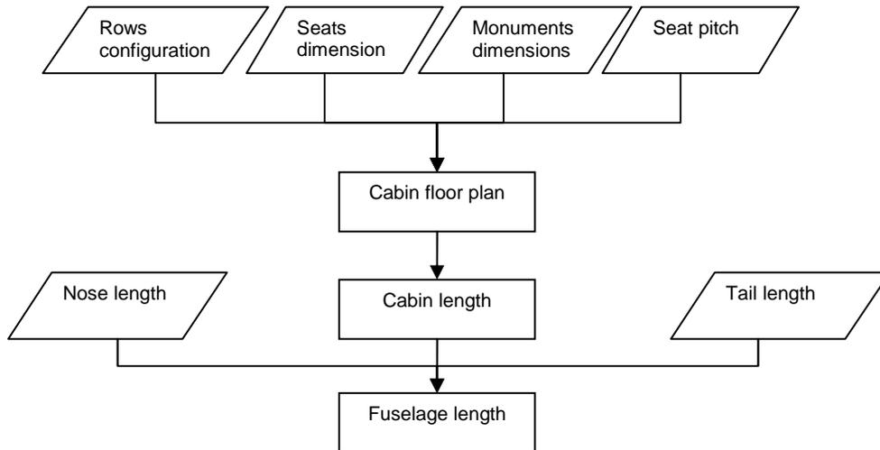
**Fig. 1.20 Calculation of cabin and fuselage length**
