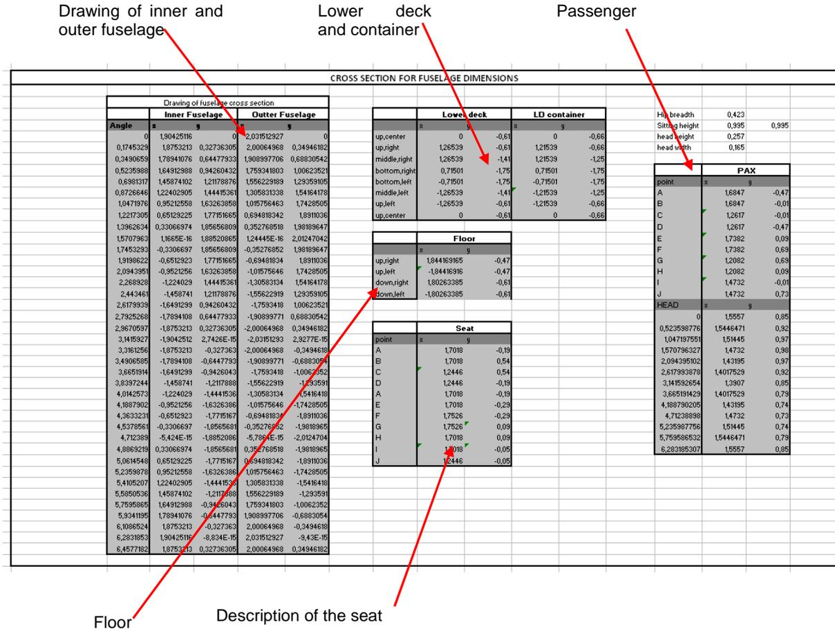
**Fig. 2.32 Overview of the calculations for cross section drawing**
