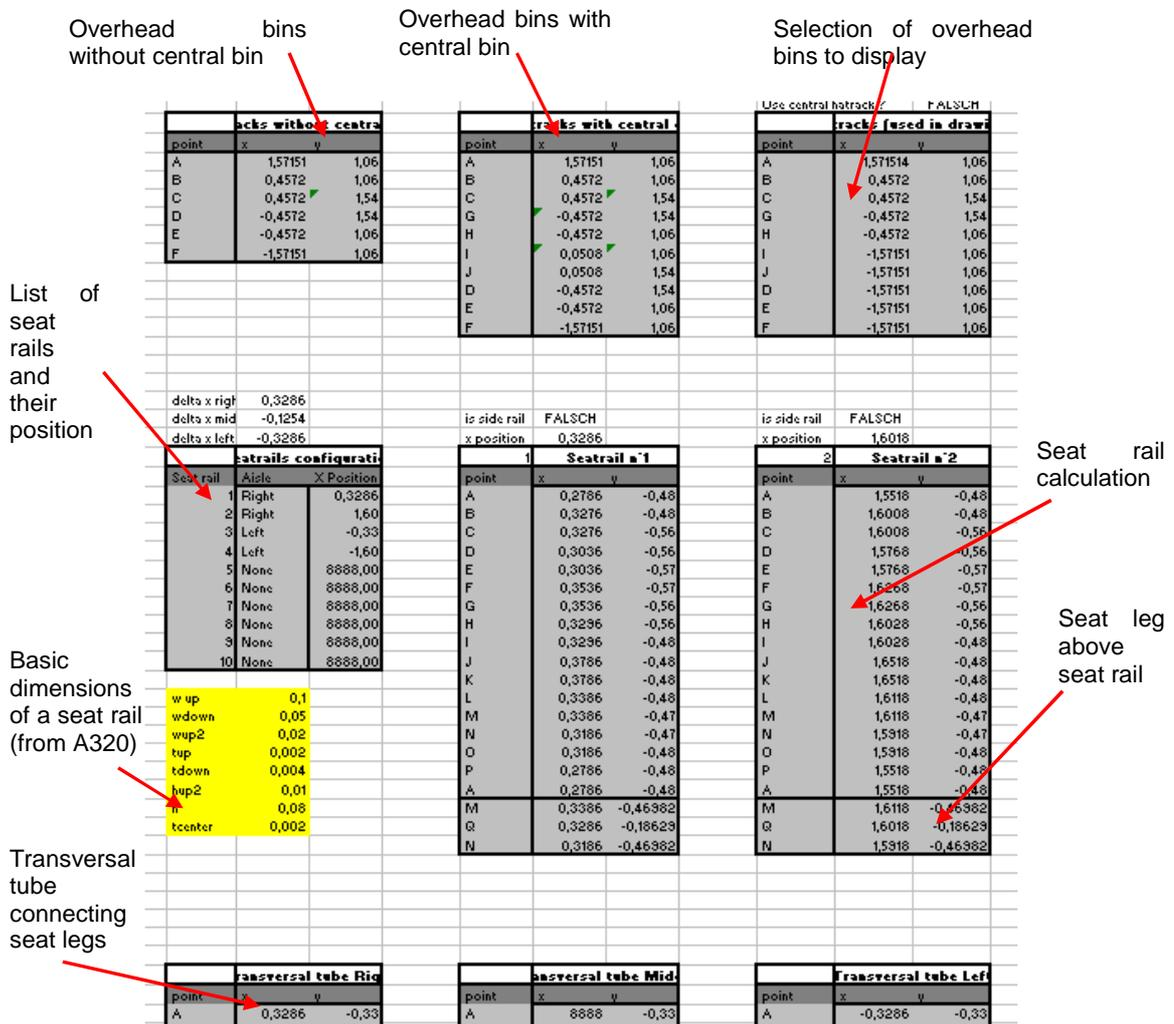
**Fig. 2.38 Calculation of various items coordinates for cross section display**
