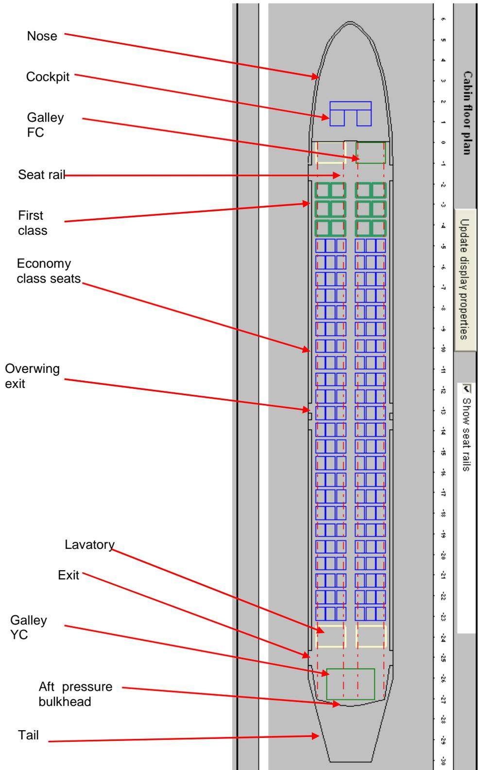
**Fig. 2.20 Cabin floor plan display**
