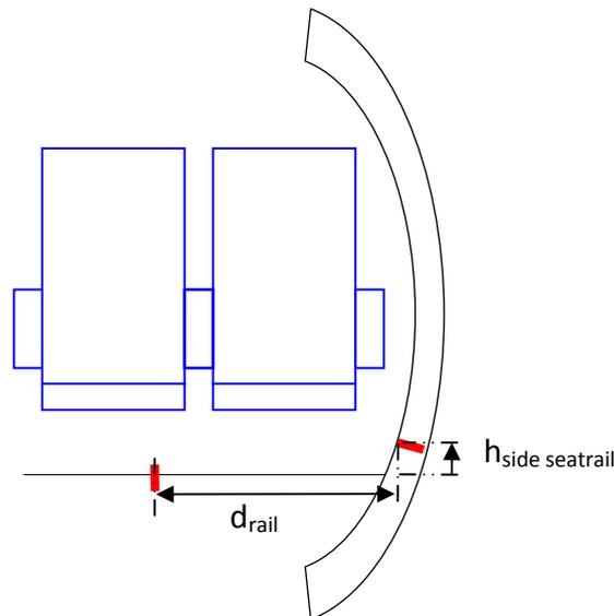
**Fig. 1.14 Positioning of side seat rails**
