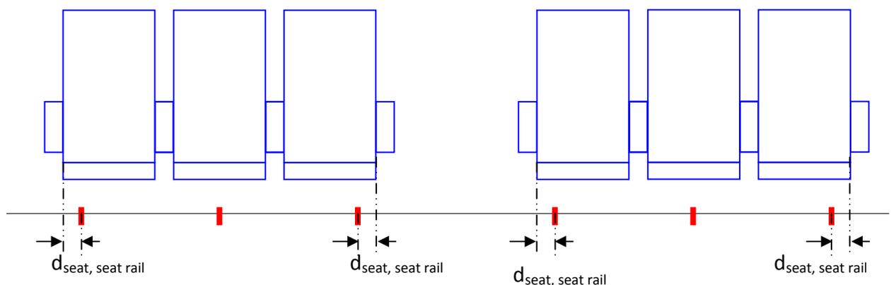
**Fig. 1.13 Positioning of seat rails on a single aisle (using symmetry)**
