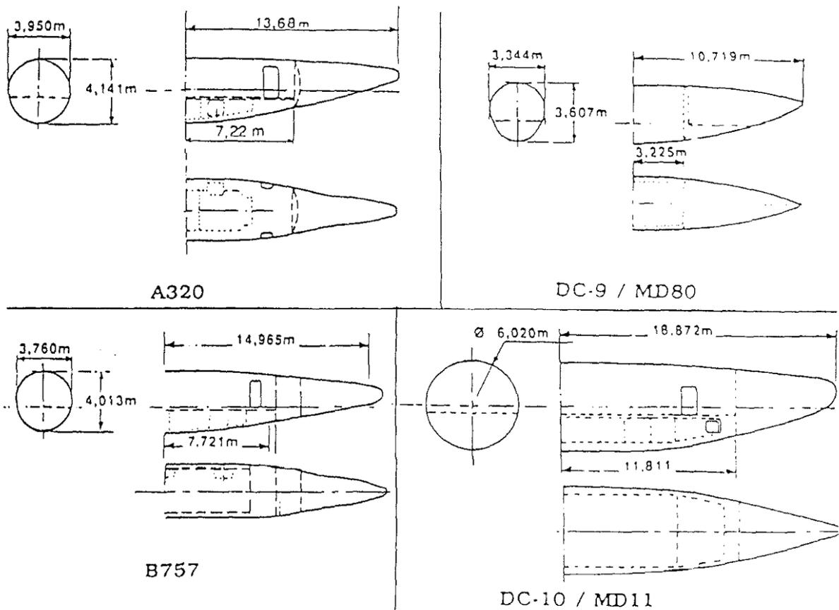
**Fig. 1.18** Tail length of existing airliners [Schmitt 1988]
