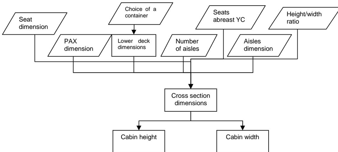
**Fig. 1.11 Calculation of cabin cross section dimensions**
