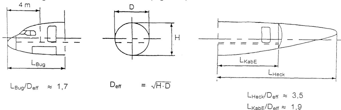
**Fig. 1.16 Nose length and tail length [Schmitt 1988]**
