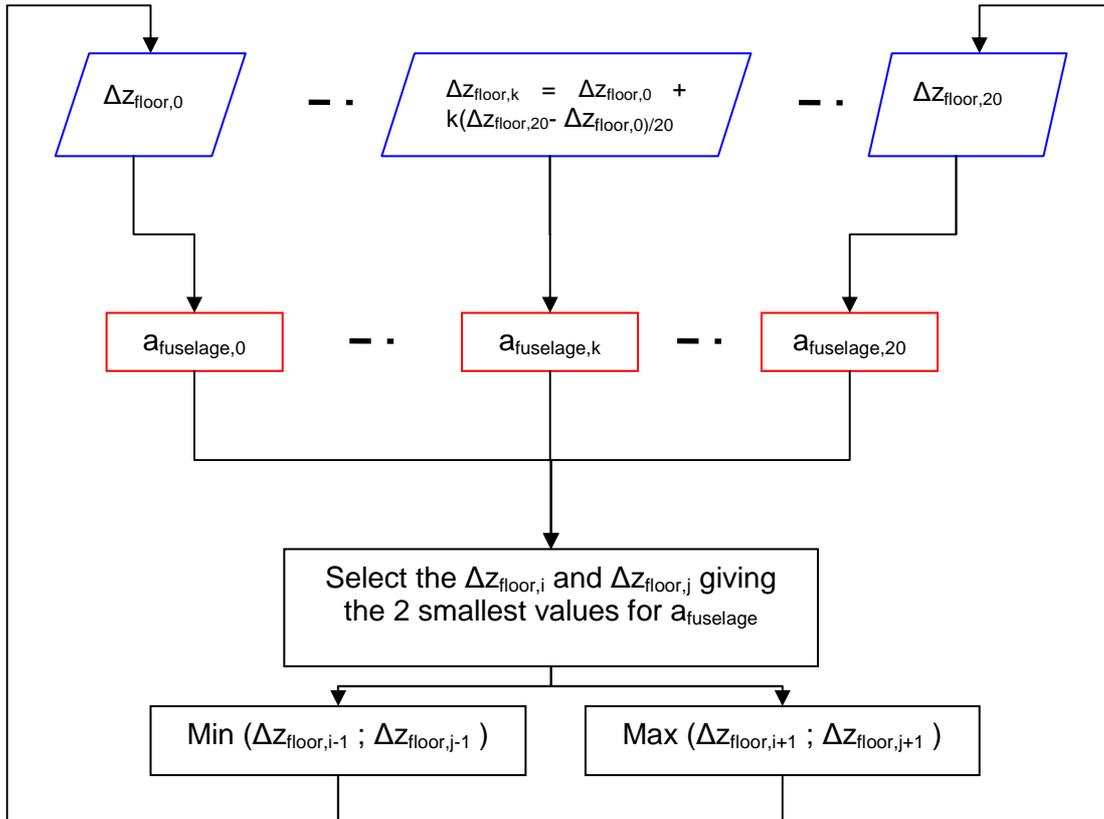
**Fig. 2.55** Loop used to find the optimal value for  $\Delta z_{floor}$
