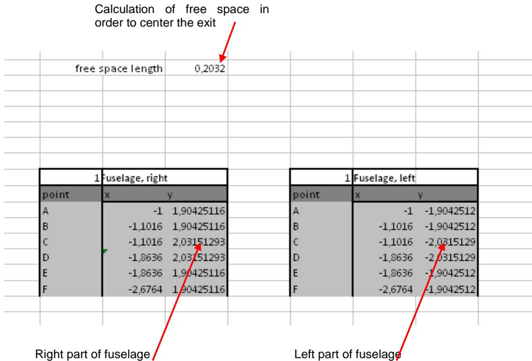
**Fig. 2.47 Calculation of fuselage parts for each row of the cabin floor plan**
