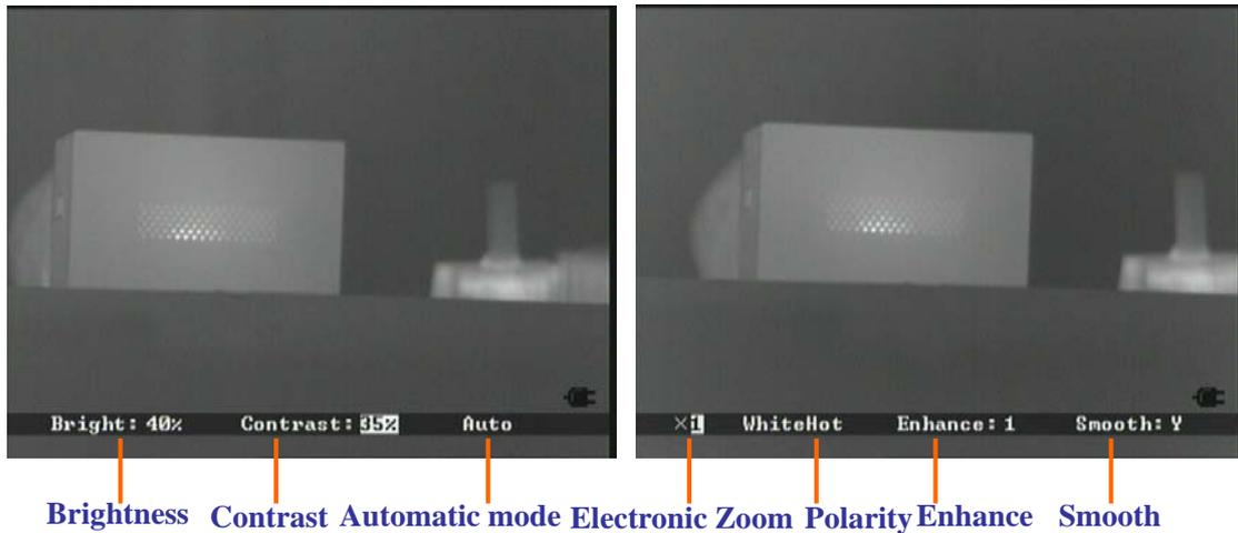
Press “M” button again to select Brightness, Contrast, Automatic Mode, Zoom, and Polarity in turn. The selected menu item will show in white on gray background. Press “+” or “-” buttons to adjust the parameters of selected item.
