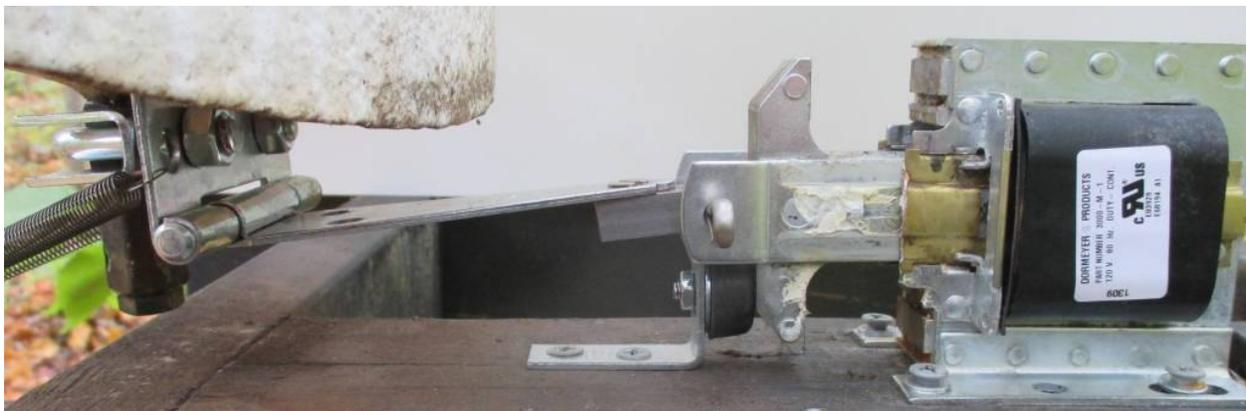
Clapper and linkage connection using the Hex Standoff protrusion.
