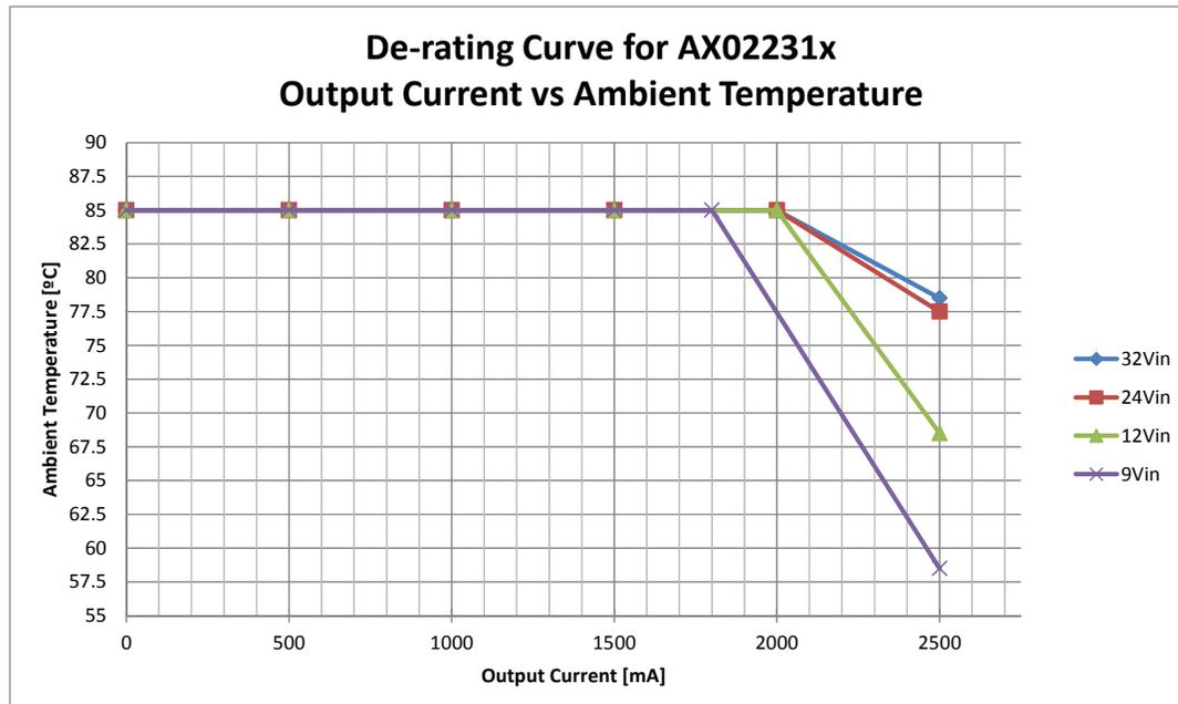
Figure 2.0 - De-rating Curve (based on both outputs on)
