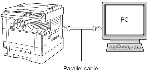
① Connecting the printer directly to your computer with a parallel cable ..... **Page 5**
