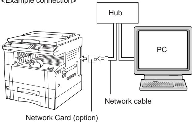
① Connecting a network cable (100Base-TX, 10Base-T, etc.) to the printer ..... **Page 5**
