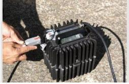
9) Plug ballast in to power source. Bulb ignites in around 0 – 200 seconds.
