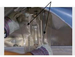
3) Grip bulb at top and unscrew slowly and carefully by turning to the left. Pull out bulb.
