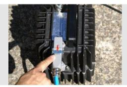
**Attention:** Always make sure to connect to existing and running power sources. Interruptions and gaps in electricity flow may cause delays in ignition of bulb or even result in its damage.
