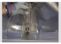
4) Insert new bulb by screwing it to the right in to socket. Make sure it sits correct, firm.
