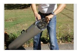
3) Place POWERMOON® with bottom pin on solid ground. Grip black handle bar, pull pin and press down until POWERMOON is fully opened and locked in place.
