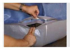
2) Open upper screw of burst cage, then bend burst cage until hand can get through to grip bulb.
